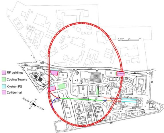
Figure 4: The new SuperB accelerator complex at one of the possible sites, the Frascati National Laboratory.
