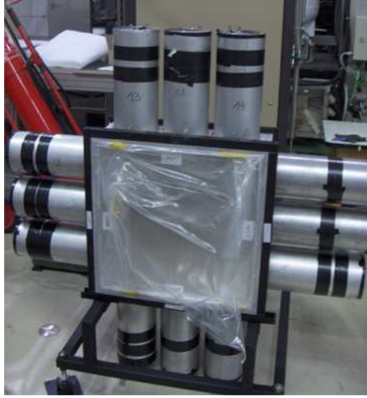
Figure 2.14: Aerogel-Čerenkov detector [44]. Twelve photomultiplier tubes are located at the narrow sides of the quadratic box containing the aerogel radiator.
