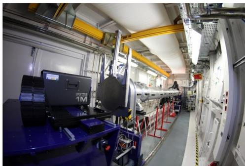
Figure 3: SAXS detector and flight tube in the End Station.
