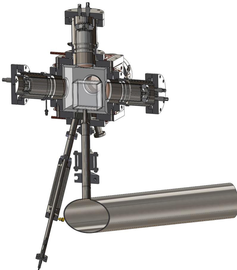
Figure 8.17. This CAD drawing shows a cross section of the UCNb experiment in one of the proposed 2012 geometries. Inside is shown the  $\text{CaF}_2$  scintillator with a  $\text{MgF}_2$  coating.
