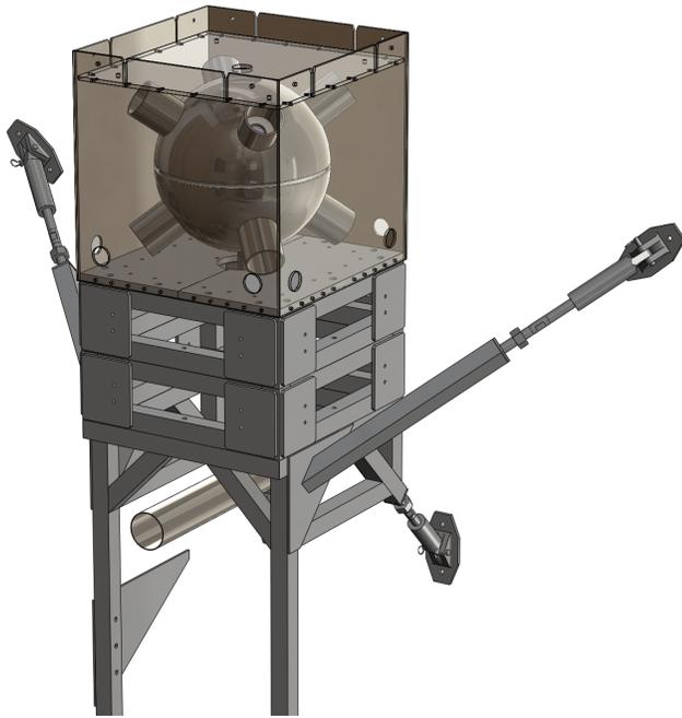
Figure 9.1. This drawing shows a cartoon of a possible upgrade of the UCNb experiment. There are eight PMTs that lie on the faces of a virtual icosahedron that lay on the outer spherical vacuum jacket.
