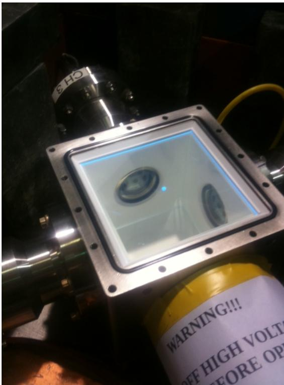
Figure 8.2. This photo shows the  $\text{MgF}_2$  polystyrene scintillator box assembled and placed inside the integrating cube. The top is on top of the box showing the insert hole for the insertable source.
