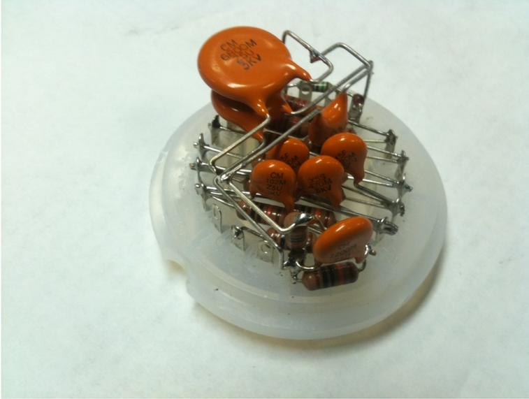
Figure 8.7. This photo shows our custom Hamamatsu R7725 base assembly.
