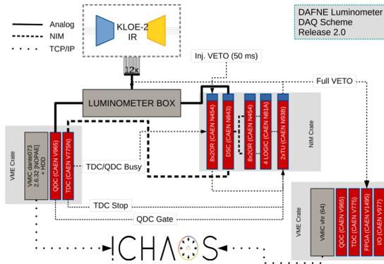
Figure 2: Schematic view of the DAQ acquisition. The signals coming from a corresponding sectors on the two sides are compared with a fixed threshold and used to measure arrival time and integrated charge when the trigger logic condition is fulfilled.
