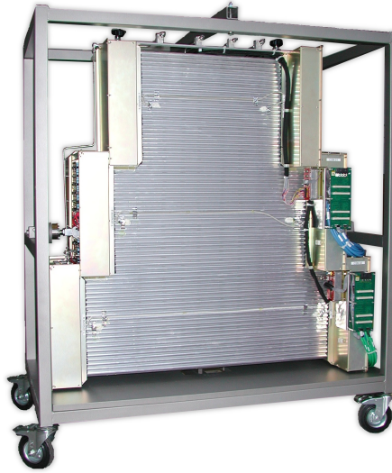
Figure 2.21: The sMDT prototype chamber mounted in a transport frame.
