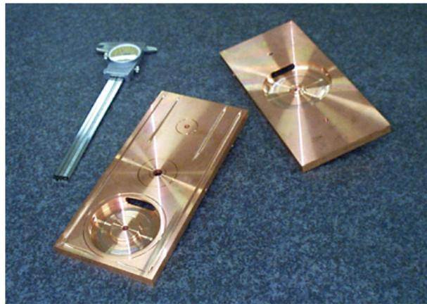
FIGURE 2.13. Half-cell-plates showing a coupling half cell (left) and an accelerating half cell (right). Note the coupling slot.
