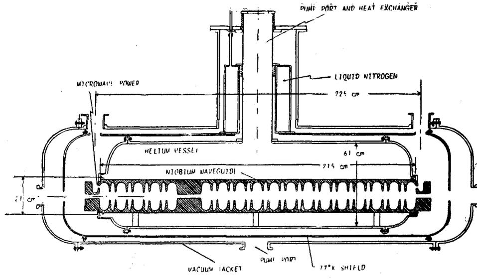
Fig. 3. General plan of the cryostat.
