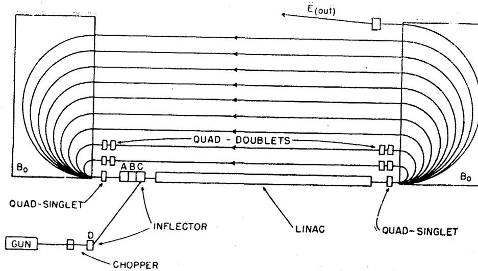
Fig. 1. Schematic microtron arrangement.
