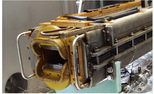
Figure 15: 4KDP6a dipole (connection side).
