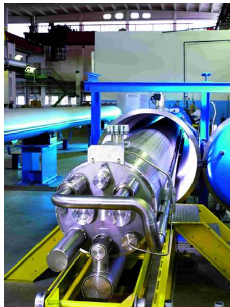
Figure 1: LHC main dipole manufacturing at BNG
