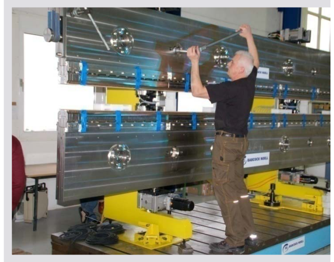
Figure 4: Assembly of a 5m long undulator prototype for XFEL
