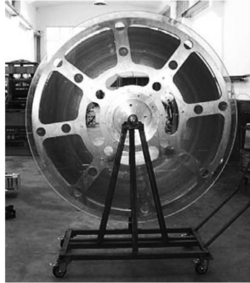
Fig. 2. 1.6 km standard stabilized multifilamentary MgB_2 tape in only one piece.
