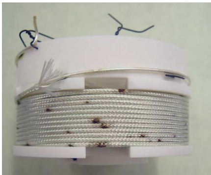
Figure 3: Intermittent leakage on the surface of the mullite-braid-insulated wire after reaction of test coil 3.
