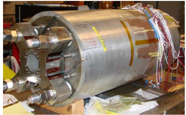
Figure 15. Photo of a completed TQS quadrupole. The four thick rods provide the strong axial support.
