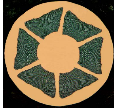
Fig 3: Double stack wire with innovative sector geometry (photo courtesy of European Advanced Superconductors)
