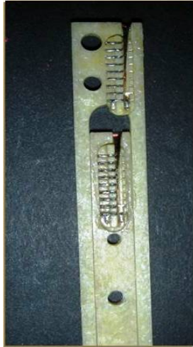
Figure 1: Prototype quadrupole-compensated harmonic coil for Linac4 permanent magnets.
