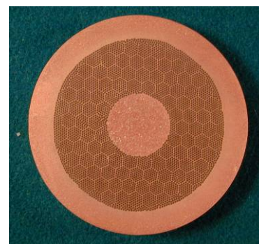
Figure 3: The Nb-Ti strand for ITER PF1&6 coils. Strand diameter: 0.73 mm, Cu/nonCu ratio: 1.6, filament diameter: 6.8 \mu\text{m} .
