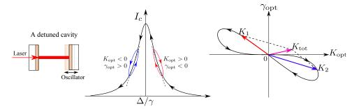
Figure 1.5 – Plot showing the optical spring effect in a detuned optical cavity. The radiation pressure is proportional to the intra-cavity power which depends on the position of the test mass. The non-zero delay in the cavity response gives rise to an (anti-)damping force. By injecting two laser beams at different frequencies, this creates a double optical spring and the system can be stabilized (right panel).
