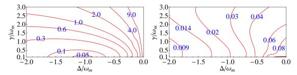
**Figure 7.1** – A contour plot of the occupation number as a function of cavity bandwidth  $\gamma$  and detuning  $\Delta$  for the unconditional state (left) as obtained in Refs. [44, 45] and optimally controlled state (right), for which the details are in Secs. 7.4, 7.5, 7.6.
