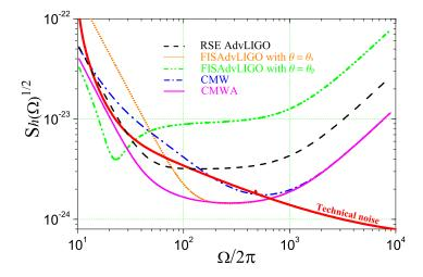
$\begin{tabular}{ll} {\bf Figure~3.4}-{\bf Quantum-noise~spectrums~of~different~schemes~using~the~same}\\ {\bf parameters~as~the~optimal~CMWA~to~show~how~different~parameters~affect~sensitivity~of~the~CMWA~scheme.} \end{tabular}$
