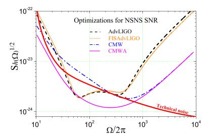
**Figure 3.2** – Quantum-noise spectra of different schemes with optimized parameters for detecting gravitational waves from NS-NS binaries. The optimal values for the parameters are listed in Table. 3.2.
