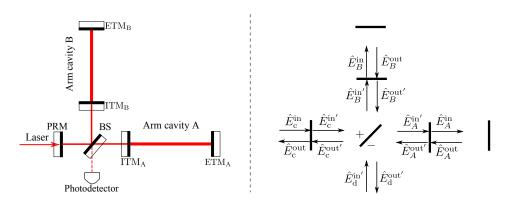
Figure 2.11 – A schematic plot of a Michelson interferometer with a power-recycled mirror (PRM) and additional ITMs to form arm cavities (left). The corresponding propagating fields are indicated in the right diagram.
