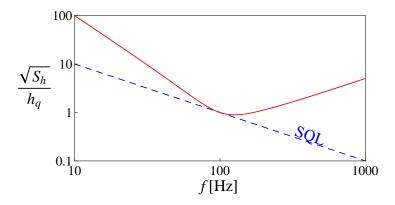
Figure 2.12 – The GW strain-referred sensitivity of an advanced GW detector with power-recycled mirror and arm cavities, given the specifications detailed in the main text. Here, we have normalized the spectrum by  $h_q$ , which is defined to be  $h_{\rm SOL}$  at 100 Hz.
