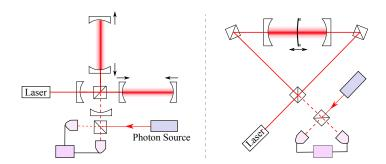
Figure 10.1 – Possible experimental schemes: (i) an interferometric gravitational-wave detector with kg-scale test masses (left) [72] and (ii) A tabletop coupled cavity scheme with a ng-scale membrane (right) [31].
