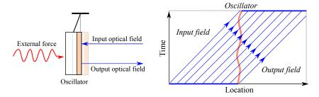
**Figure 1.2** – A schematic plot of an optomechanical system (left), and the corresponding spacetime diagram (right). The output optical field that contains the information of the oscillator motion is measured continuously by a photodetector. For clarity, the input and output optical fields are placed on opposite sides of the oscillator world line.
