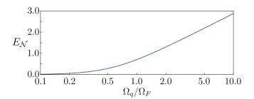
Figure 8.2 – Logarithmic negativity  $E_{\mathcal{N}}$  as a function of the ratio  $\Omega_q/\Omega_F$ . A mechanical quality factor  $Q_m = 10^3$  is chosen.
