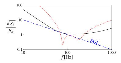
**Figure 2.15** – The GW strain-referred sensitivity of a signal-recycling GW detector given a phase-quadrature detection  $\zeta = \pi/2$ . The solid curve corresponds to the RSE scheme with  $\theta = \pi/2$  and  $\sqrt{R_S} = 0.6$ . The dashed curve shows the case with  $\theta = 1.1$  and  $\sqrt{R_S} = 0.9$ .
