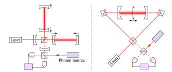
Figure 1.7 – Possible schemes for preparing non-Gaussian quantum states of mechanical oscillators. The left panel shows the schematic configuration similar to that of an advanced GW detector with kg-scale suspended test masses in both arm cavities. The right panel shows a coupled-cavity scheme proposed in Ref. [31], where a ng-scale membrane is incorporated into a high-finesse cavity. In both cases, a non-Gaussian optical state is injected into the dark port of the interferometer.
