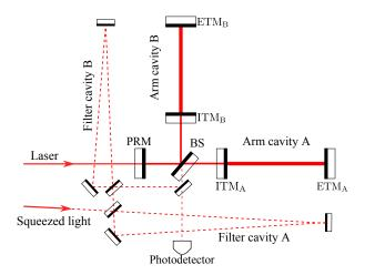
Figure 2.17 – A schematic plot of the frequency-dependent squeezed input configuration. A frequency-independent squeezed light, filtered by two detuned Fabry-Pérot cavities in sequence, produces the required frequency dependence.
