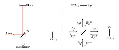
**Figure 2.10** – A schematic plot of a simple Michelson interferometer (left); and its mathematical model with propagating optical fields (right).
