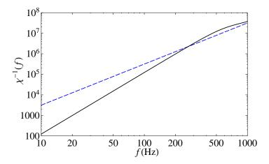
**Figure 4.1** – The resulting response function with a double optical spring (solid), compared with that of a free mass (dashed).
