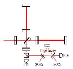
Figure 1.4 – A schematic plot showing the double-squeezed input configuration of an advanced GW detector. Two frequency-independent squeezed (SQZ) light are filtered by a tuned Fabry-Pérot cavity before being injected into the dark port of the interferometer. Two photodetections (PD) are made, at both the filter cavity, and at the interferometer outputs, to maximize the sensitivity.
