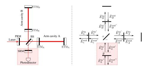
Figure 2.13 – A schematic plot of a Michelson interferometer with a power-(PRM) and signal-recycled mirrors (SRM) and additional ITMs to form arm cavities (left). The corresponding propagating fields are indicated in the right-hand diagram, with  $\theta$  being the detuned phase.
