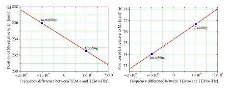
**Figure 6.10** – Panels (a) and (b) show the mode gap between  $TEM_{10}$  and  $TEM_{00}$  as a function of position of  $M_0$  relative to  $L_1$  and position of  $L_1$  relative to  $M_1$  respectively. The dots in both figures are the situations considered in Fig. 6.9. Clearly, we can tune between the instability and cooling regimes continuously.
