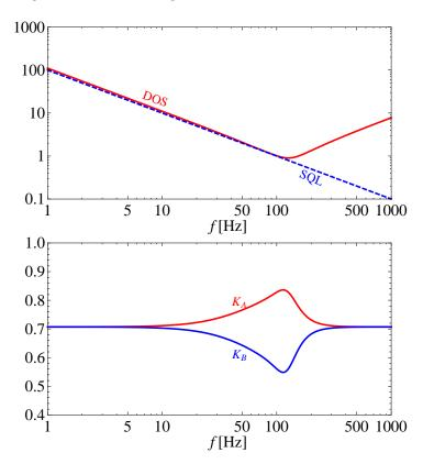
**Figure 4.2** – The top figure shows the DOS noise curve normalized with respect to the standard quantum limit at 100 Hz. The bottom one shows the corresponding optimal kernel functions for the two carriers.
