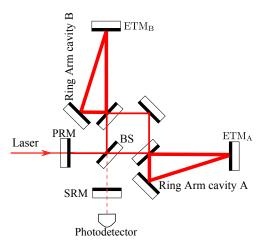
Figure 2.24 – A schematic plot of a Sagnac-type speed meter configuration.
