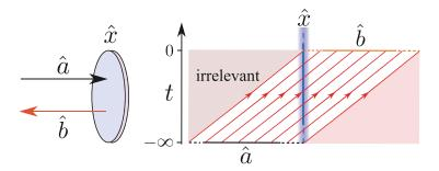
Figure 8.1 – A schematic plot of the model and the corresponding spacetime diagram. Here  $\hat{x}$ ,  $\hat{a}$  and  $\hat{b}$  denote the oscillator position, ingoing and outgoing field respectively. For clarity, we intentionally place  $\hat{a}$  and  $\hat{b}$  on different sides of the oscillator world line. The tilted lines represent the light rays. The optical field entering after the moment of interest (t=0) is out of causal contact, and thus irrelevant.
