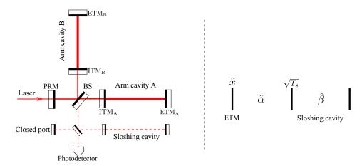
**Figure 2.22** – A schematic plot of a speed-meter configuration with coupled cavities. A sloshing cavity is added after the dark port. Such a configuration can be mapped into a three-mirror cavity as schematically shown in the right-hand panel, forming a pair of coupled cavities.
