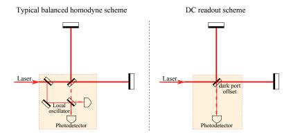
Figure 2.5 – A schematic plot of two homodyne readout schemes.
