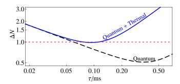
**Figure 9.2** – The resolution  $\Delta N$  for measuring mechanical energy quantization depending on the integration duration  $\tau$  with total noise (Solid) and quantum noise only (Dashed).
