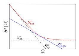
**Figure 2.1** – A schematic plot of the displacement noise spectrum for a typical interferometer. Increasing or decreasing the optical power, the power-independent lower bound of the total spectrum will trace over the SQL.
