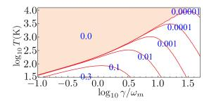
Figure 7.8 – Logarithmic negativity  $E_N$  as a function of cavity bandwidth and environmental temperature. We have chosen  $\Omega_q/\omega_m = 1$ ,  $\Delta = 0$ ,  $Q_m = 5 \times 10^5$  and  $\omega_m/2\pi = 10^6$  Hz. The shaded regimes are where entanglement vanishes.
