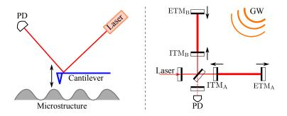
**Figure 1.1** – A schematic plot of an atomic-force microscope (left), and a gravitational-wave (GW) detector (right).
