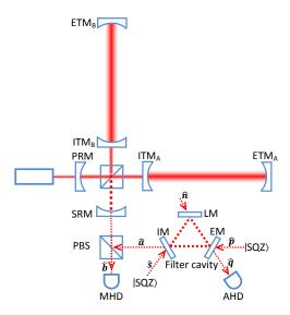
Figure 3.1 – Schematic plot of the proposed configuration. Two squeezed light beams  $\hat{s}$ ,  $\hat{p}$  are injected from both side of the filter cavity rather than the one which was considered in Refs. [7, 70]. The signal is detected by the main homodyne detector (MHD) and an additional detector (AHD) is placed at the idle port of the filter cavity.
