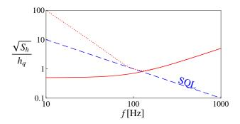
**Figure 2.20** – The GW strain-referred sensitivity of a variational-readout scheme (solid curve). The low-frequency back-action noise is completed evaded, thus achieving a sensitivity limited only by shot noise.
