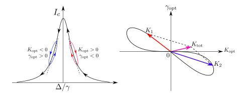
Figure 2.21 – The optical power as a function of cavity detuning  $\Delta$  (left). A double optical spring,  $K_{\text{tot}}(\Omega) = K_1(\Omega) + K_2(\Omega)$ , which has both positive rigidity and damping (right). The black curve (right) shows a parametric plot of the optical spring  $K(\Omega)$  as a function of detuning.
