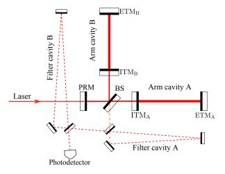
**Figure 2.19** – A schematic plot of the variational-readout configuration. The output is filtered by two detuned Fabry-Pérot cavities before the detection.
