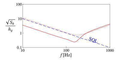
Figure 2.23 – The GW strain-referred sensitivity of the speed meter scheme shown in Fig. 2.22. We have chosen  $\gamma/2\pi = 210$  Hz,  $\omega_s/2\pi = 180$  Hz and  $I_c = 800$  kW. The dotted curve is the case without a phase-squeezed input, and the solid curve has  $e^{-2q} = 0.1$  (a 10 dB squeezing).
