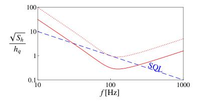
Figure 2.18 – The GW strain-referred sensitivity of a frequency-dependent squeezing input interferometer (solid curve). The squeezing factor is  $e^{-2q} = 0.1$ . The other specification is the same as Fig. 2.12.
