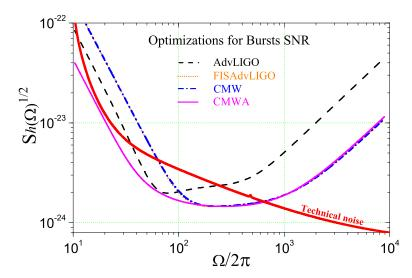
**Figure 3.3** – Quantum-noise spectra of different schemes which are optimized for detecting GWs from Bursts. The optimal values for the parameters are listed in Table. 3.3.
