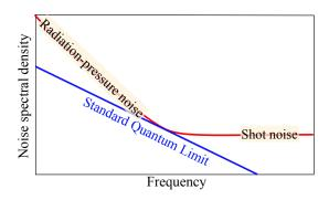
Figure 1.3 – A schematic plot of the displacement noise spectral density for a typical GW detector. When we increase the power, the shot noise will decrease and the radiation-pressure noise will increase, and vise versa. The locus of the power-independent lower bound of the total spectrum defines the SQL (blue).
