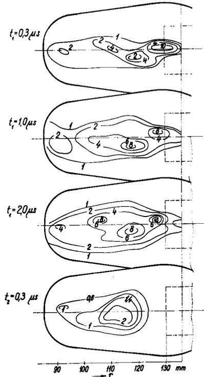
**Fig. 3** Distribution of charge density across the cross-section of the vacuum chamber at different times  $t_1$  after the beginning of the injection pulse and at a time  $t_2 = 0.3 \mu s$  after the end of the injection pulse.
