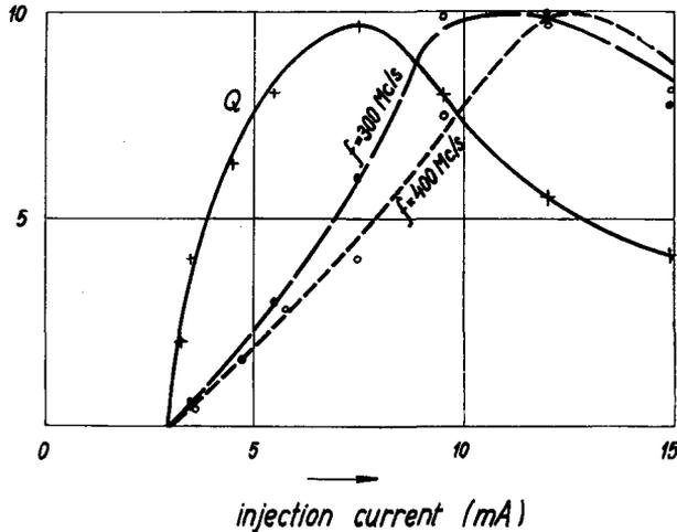
Fig. 2 Full curve (Q) represents the dependence of the captured charge on injection current. Dashed curves represent the dependence of the square of oscillation amplitude for 2 oscillation modes ( $f = 300$  Mc/s,  $f = 400$  Mc/s) on injection current.
