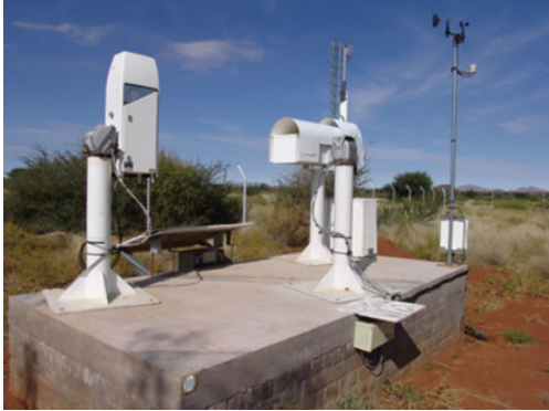
Figure 3. Picture showing the Ceilometer (left, this device is no longer on site), the weather station (right) and the scanning radiometer (in front of the weather station).
