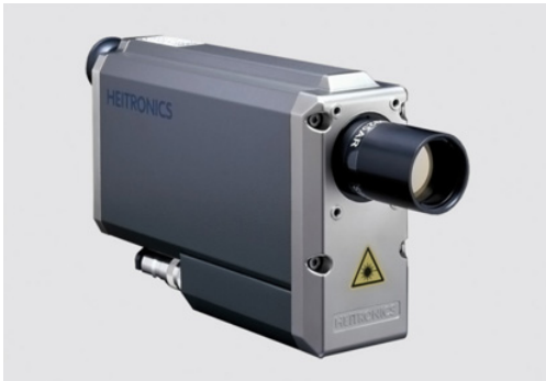
Figure 4. The Heitronics KT19.82 IR radiometer. Five of these devices are operated on the H.E.S.S. site for monitoring primarily clouds and aerosols.
