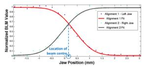
Figure 3: One example of the alignment fits generated for the beam-based setup with the left (L) and right (R) jaws.
