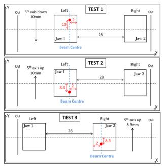
Figure 2: Schematic diagrams for Test 1, Test 2 and Test 3. The impact location is shown in red and all dimensions are in mm.
