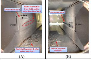
Figure 6: Preliminary visual inspection. (A) Damage on the left jaw caused mainly by Test 1 beam impact. (B) Damage on the right jaw caused by Test 3 beam impact.
