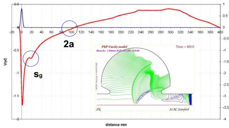
Figure 7: Wake potential of the PEP-II cavity for a 1.8 mm bunch.
