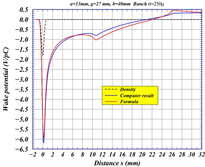
Figure 2: Comparison of the analytical and numerically computed wake potentials.
