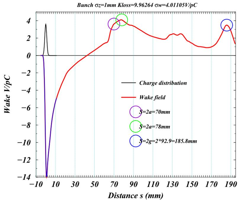
Figure 6: Wake potential of the TESLA cavity.
