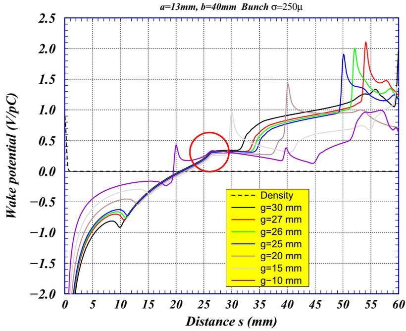
Figure 5: Peaks in wake potentials at the distance, equal to double size cavity gap.
