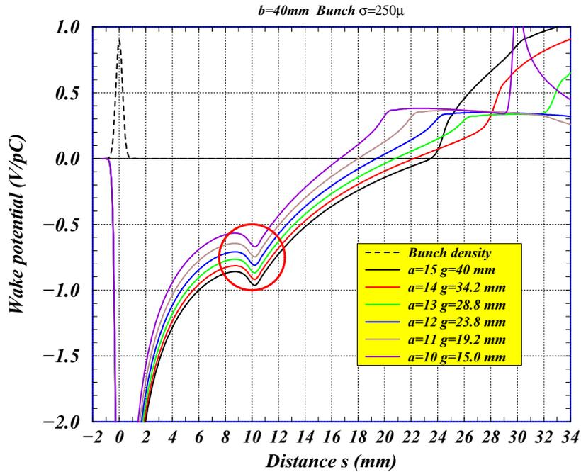
Figure 4: Wake potentials of cavities of the fixed time flight.
