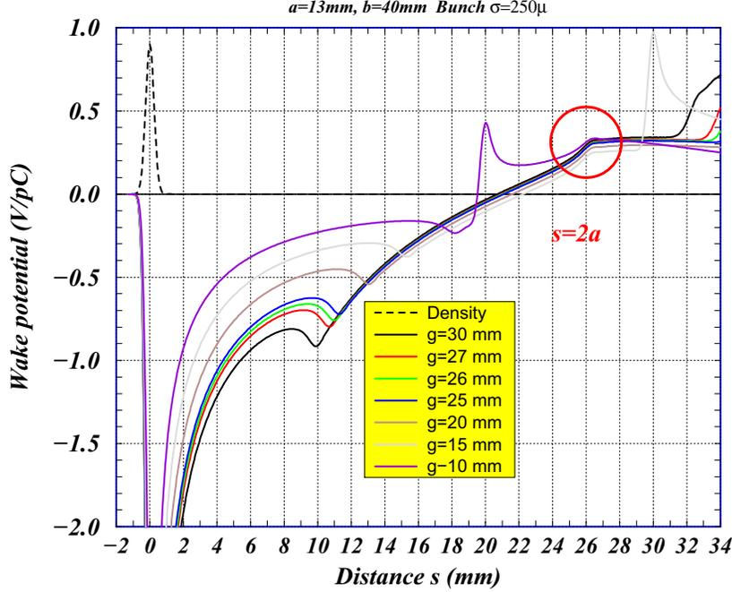
Figure 3: Wake potential of cavities of different gap size, but fixed radius of aperture.
