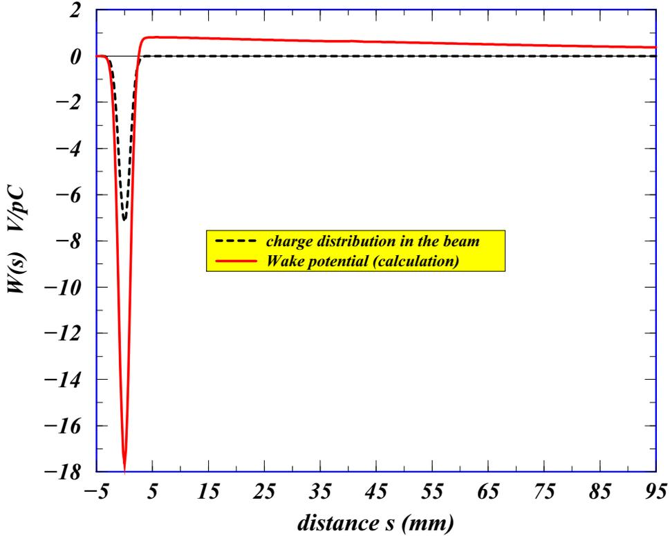
Figure 1: Wake potential of a 1 mm bunch passing an iris with a hole radius of 20 mm in a cylindrical pipe of radius of 70 mm
