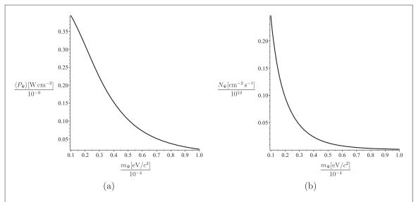
**Figure 1.** The average ALP energy flux density (40) and average ALP flux density (42) versus the ALP mass  $m_\Psi$  for the parameters  $\omega_p=2\pi\times 10^{13}~{\rm rad~s^{-1}}, \gamma=100, B=35~{\rm T}, g=0.66\times 10^{-10}~{\rm GeV}^{-1}$ .
