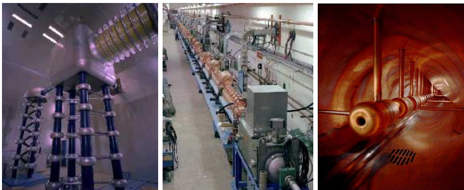
Figure 4.3: Cockroft-Walton and the Linac
