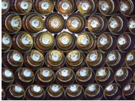
**Figure 2.30:** The arrangement of HPDs in the upper box of RICH1.
