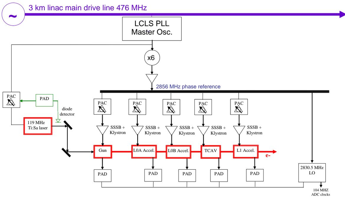
Figure 2: Low level RF for the LCLS photoinjector.
