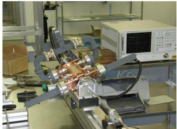
Fig.4. The plunger set-up for nodal measurements.
