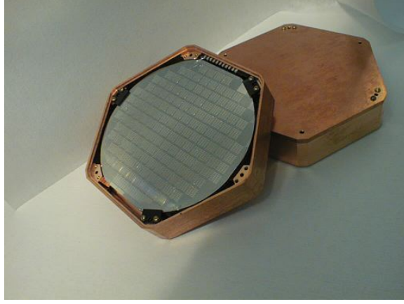
Figure 3.1: A Z-dependent Ionization and Phonon (ZIP) detector, showing the photolithographic patterning of the phonon sensors.
