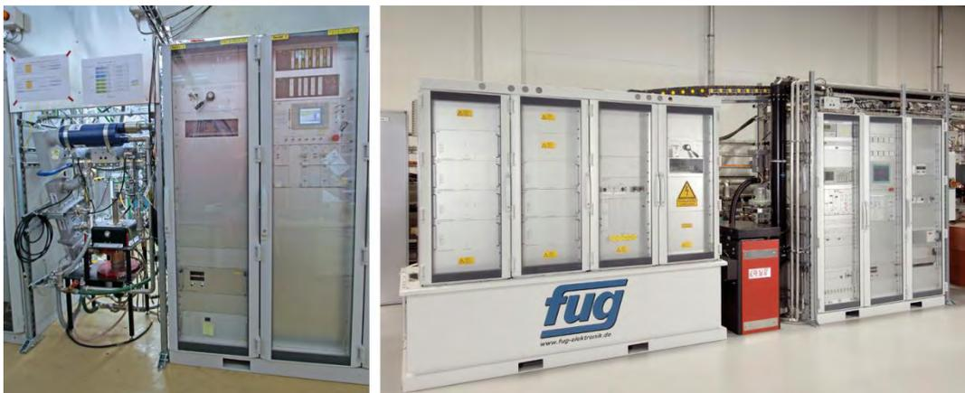
Figure 10.9. Example of two IOT based transmitters. On the left is a 30 kW, 1.3 GHz system operated at the HoBiCaT facility at the Helmholtz-Zentrum Berlin. On the right is an 80 kW, 500 MHz transmitter operated at the MLS. [[10.15]; Adapted under Creative Commons Attribution 3.0 License ([www.creativecommons.org/licenses/by/3.0/us/](http://www.creativecommons.org/licenses/by/3.0/us/)) at [www.JACoW.org](http://www.JACoW.org).]
