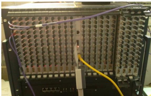
**Figure 6:** Photo of the new DAQ electronics: The system consists of 20 front-end modules each processing the signals from 3 bolometers, and a readout module (in the center) for generation of a central trigger and with a PCI Express (PCIe) interface.
