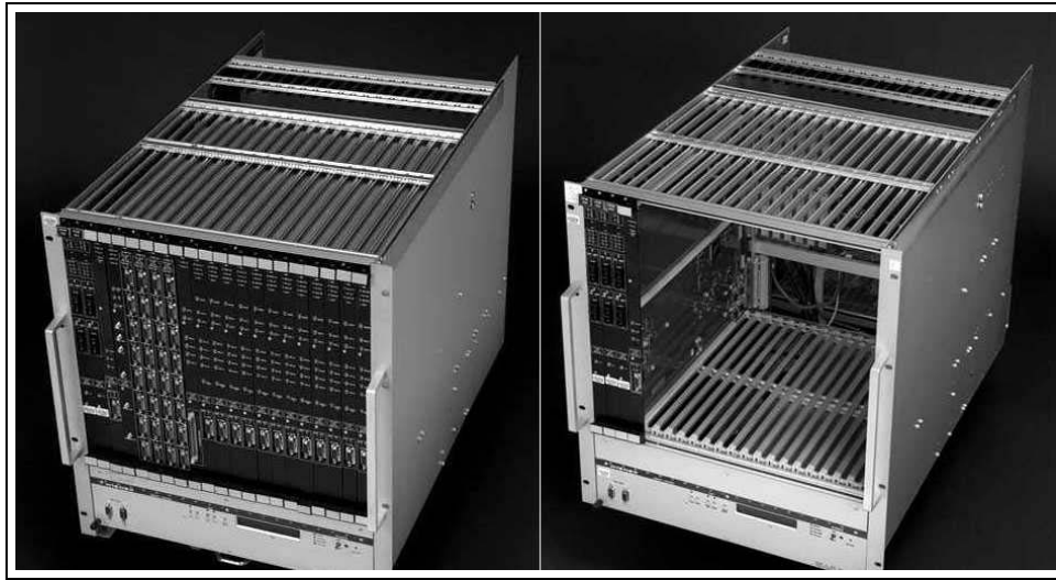
Figure 4.13: (left) A fully populated Master Crate, (right) A Slave Crate showing DAQ system hardware installed
