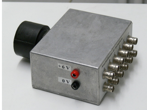
Figure 3.4: Box to supply the hydrophones with the required 6 V supply voltage and to readout their differential signals.
