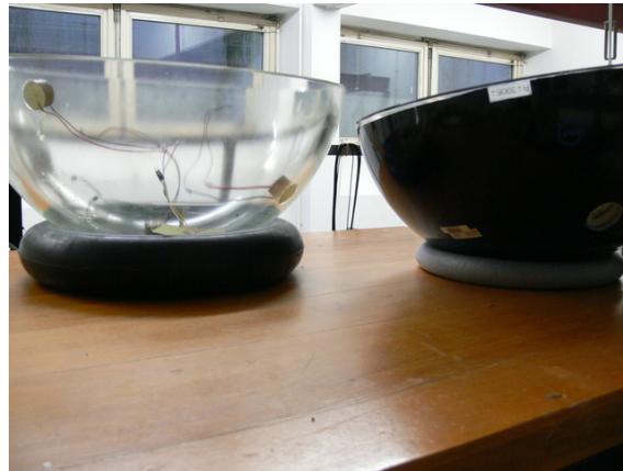
Figure 11.5: Hemispheres placed next to each other on an airtube and rubber foam.
