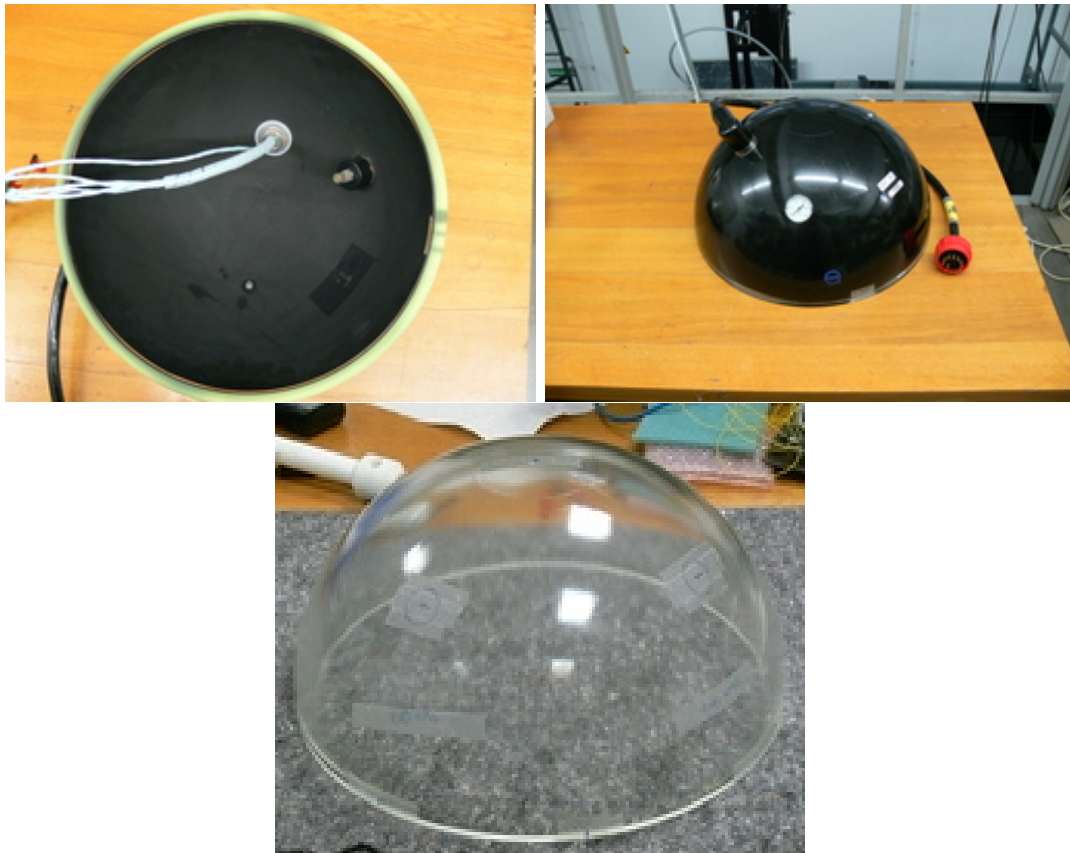
Figure 6.1: Photograph of the two hemispheres of a Vitrovex sphere:
