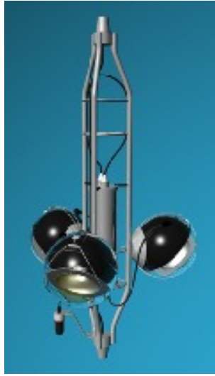
Figure 1: Schematics of an ANTARES optical storey. The three OMs are connected to the titanium cylinder in the centre of the scheme.
