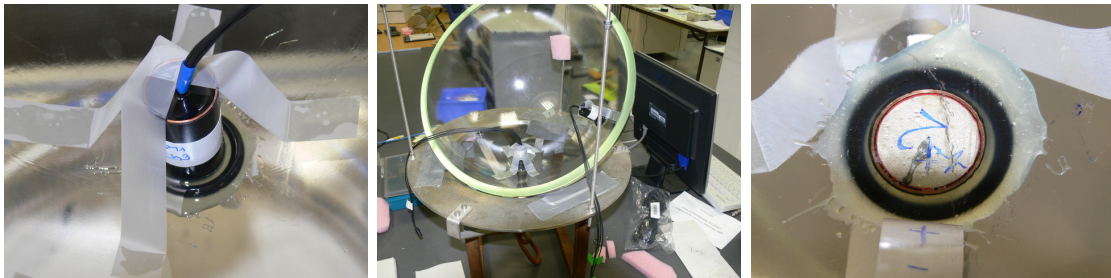
Figure B.8: Finished sensors glued to the hemisphere and quality check through the glass.
