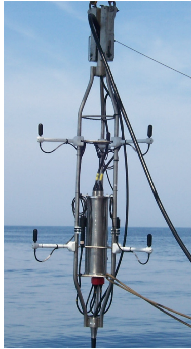
Figure 3.8: Photograph of an OMF supporting hydrophones. The white hydrophone supports are the same as used in the hydrophone calibration.
