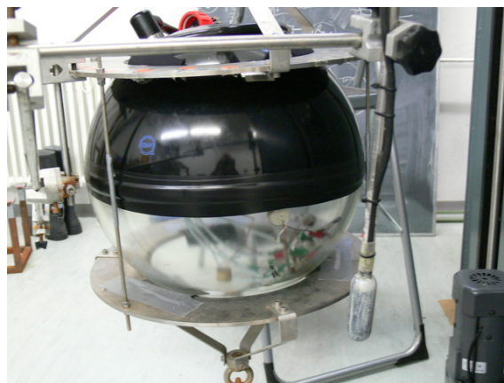
Figure 10.7: Complete test setup with the radial distance of the emitter from the sphere scaled down with respect to the distance used for the measurement.
