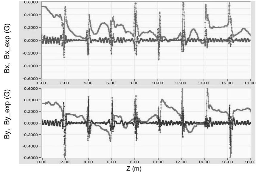
**FIGURE 3.** Transversal Magnetic Field in CS at  $B_z=100\text{G}$  (light color – Initial with compensation coils off, dark color – after compensation by dipole correctors).
