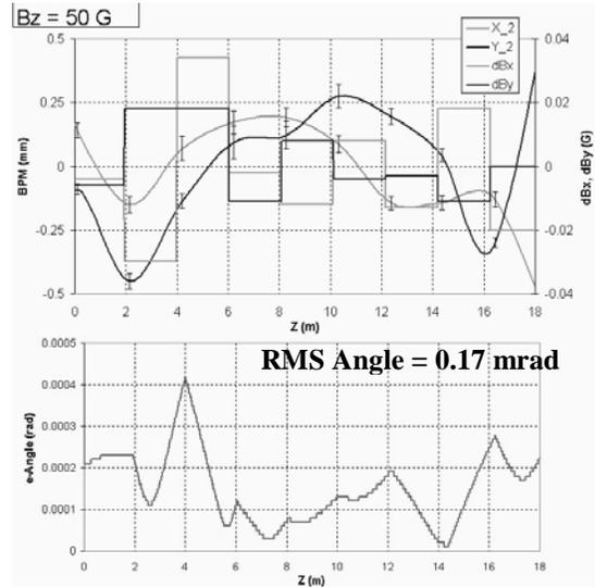
**FIGURE 7.** BPM readings (error bars) & their fits (solid curves) after dipole settings were recalculated for Bz =50G. Beam angles and offsets at the CS entrance:  $\theta_x = -0.2 \text{ mrad}$ ,  $\theta_y = -0.1 \text{ mrad}$ ,  $X_0 = 0.15 \text{ mm}$ ,  $Y_0 = -0.1 \text{ mm}$ .
