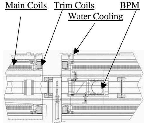
**FIGURE 1.** Cross-section of Instrumentation gap between two solenoid modules (gap shielding is not shown).
