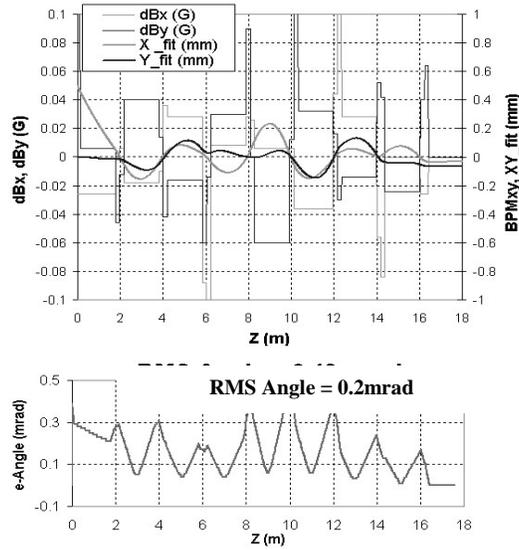
**FIGURE 5.** Simulation of beam trajectory and angle improvements after field correction in the gaps by trim dipoles only.
