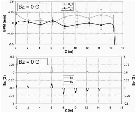
**FIGURE 6.** BPM readings (dots) & their fits (solid curves) after field correction made by trim dipoles Bx, By (bottom plot).
