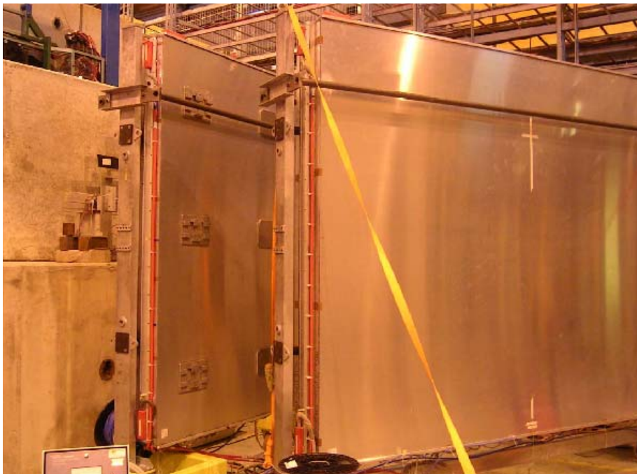
Figure 6.2: The setup used in the test-beam 2004. From left to right, it is possible to distinguish the beam trigger scintillators, the MB1 and the MB3 chambers. The muon beam was entering in the experimental hall from the concrete wall behind the scintillators.
