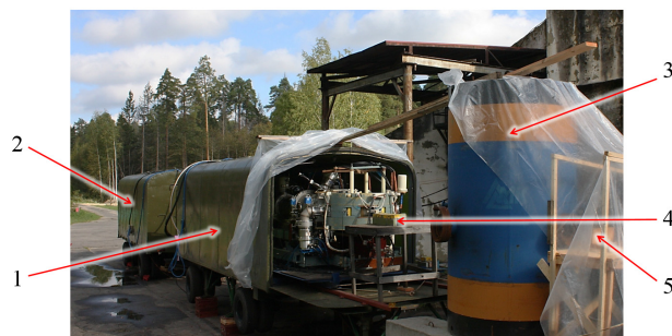
Figure 1: Photo of a single-beam three-frame mobile radiographic complex: 1 – accelerator unit; 2 – pulsed power unit of the betatron electromagnet; 3 – EPC; 4 – X-ray collimation system; 5 – shadow image recording system.
