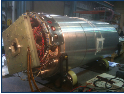
Figure 6: The cold mass of the HQ02 120 mm aperture quadrupole, designed and built by USA-LARP. This magnet, near to the final design of HL-LHC IT quadrupoles, routinely passed 12 T of peak field during power test at Fermilab. Picture taken at LBNL after structure assembly.
