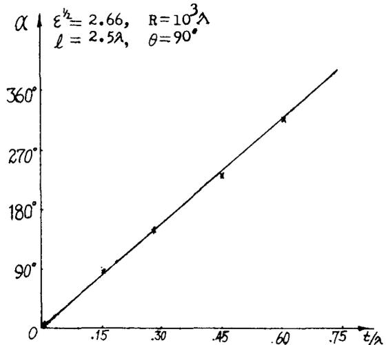
Fig. 3 - Variation of the phase delay  $\alpha$  on the axis for various of the thickness  $t$  of step.
