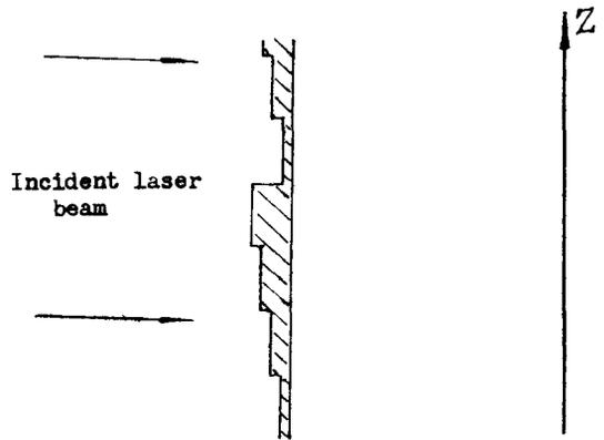
Fig. 2 - Stepwise grating (schematic) for phase adjustment, the grating and the incident laser revolving together around the Z-axis. For a four-step grating the optical path is increased by a quarter wavelength for each step.
