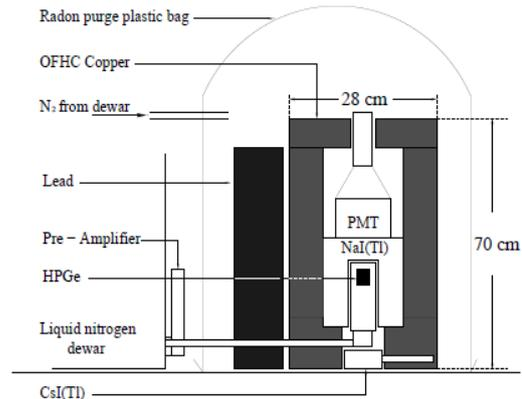
FIG. 2: Schematic drawings of the ULB-HPGe detector with its anti-Compton scintillators and passive shielding [2].
