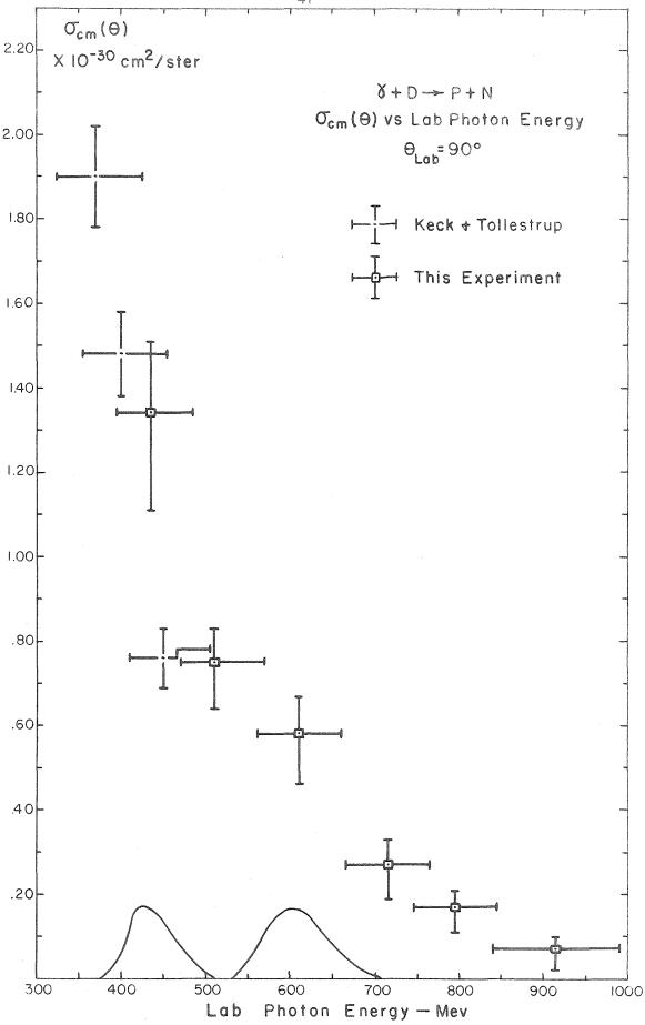
interpolation of the 93° excitation curve of Keck and Tollestrup. The horizontal error represents the photon energy interval within which lay approximately 80% of the photons which reacted to give protons detected by the telescope. The origin of the vertical error assignment is discussed in the preceding section.
