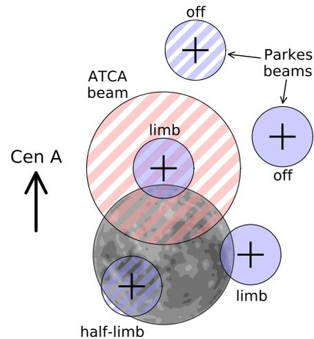
**Figure 1:** Typical pointing configuration of the Parkes beams (blue) with respect to the Moon during the 2010 Parkes-only observations and also of the ATCA beams (red) during combined observations in 2011. In the 2010 observations, the top-most ‘off’ beam was not usually used, while during 2011, the bottom-most ‘half-limb’ beam was not used. Crosses show the direction of the polarisation channels in the receivers; the overall orientation is relative to the offset from Centaurus A.
