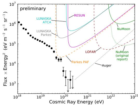
**Figure 4:** Sensitivity of prior (RESUN [15]; LUNASKA ATCA [20]; LUNASKA Parkes (these proceedings); NuMoon [6]) and future (LOFAR [21]; Parkes phased-array feed (PAF), with an assumed threshold of  $4.8 \cdot 10^{-9}$  V/m/MHz, full lunar coverage, and one week's observations) lunar searches compared to the UHE CR flux measured by Pierre Auger [7] (black points) and the UHE flux levels corresponding to no events being observed about  $3 \cdot 10^{20}$  eV.
