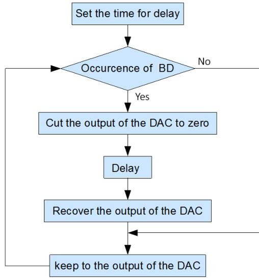
Fig. 4. (Color online) Arithmetic diagram of the interlock protection.
