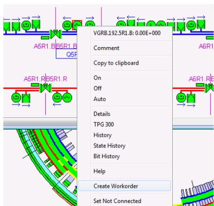
Figure 5: Work Order generation in the vacuum SCADA.
