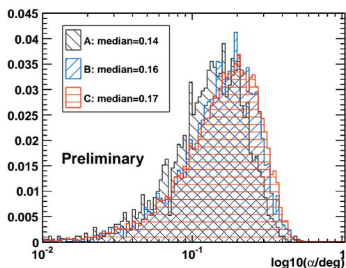
**Figure 9:** The angular difference,  $\alpha$ , between the reconstructed source position of an event and the average reconstruction position for that pulser-station orientation. The results for several different pulser orientations are shown.
