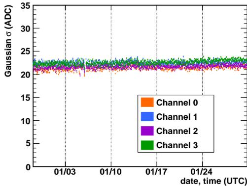
**Figure 2:** Width of the minbias triggered ADC distribution over the month of January. The width is consistent with noise from the station’s amplifiers and its lack of variation reflects the radio quiet environment of the Ross Ice Shelf.
