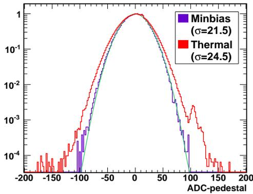
**Figure 1:** Distribution of the (sampled) waveform amplitude from one LPDA channel on the northern-most station. Randomly read out waveforms are shown by the purple, “minbias” line. Triggered event waveforms are shown by the red, “thermal” line. A Gaussian fit to the minbias data is shown by the green curve.
