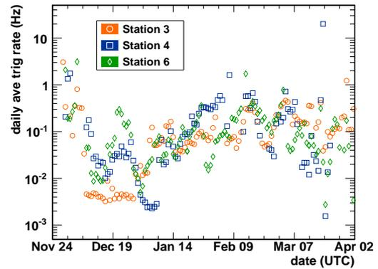
**Figure 3:** The average trigger rate of all redesigned stations in each 24-hour period since installation.
