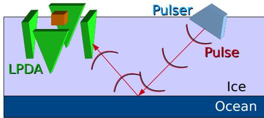
**Figure 5:** Illustration of a calibration pulse test. The radio pulse is emitted at the surface, reflects off the ice/water interface and propagates back to the surface, where it is picked up by the LPDAs at the station.
