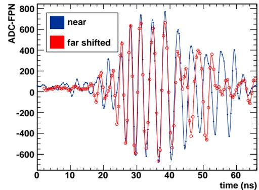
**Figure 7:** Comparison of the two waveforms from Fig. 6 after matching by shifting in time.
