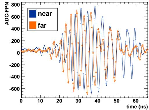
**Figure 6:** Comparison of two waveforms on one LPDA channel. The blue, “near” line with closed points shows the waveform recorded with the pulse generated at the station. The orange, “far” line with open points shows the waveform recorded with the pulse generated about 150 m from the station.
