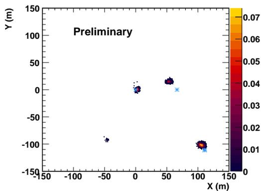
**Figure 8:** The reconstructed surface position of the pulse emission in several different signal calibration studies. Blue stars indicate an estimation of the true emission position.
