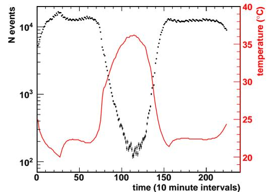
**Figure 4:** The number of events triggered on amplifier noise together with the ambient temperature, as observed in rooftop experiments at UC Irvine. The black points and left vertical axis indicate the number of triggers taken in 10 minute intervals. The red line and right vertical axis indicate the environment temperature.
