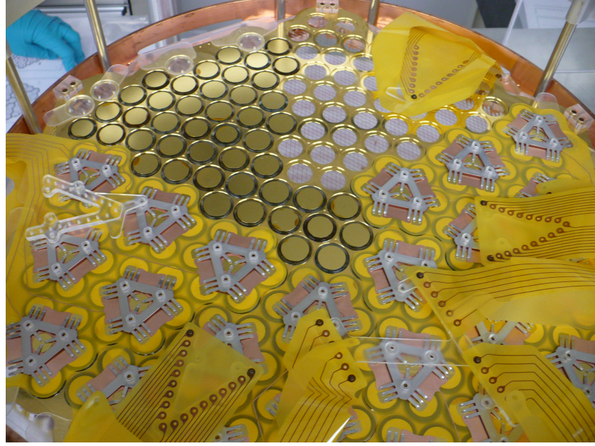
Figure 3.6.: Back (non-active) side of the light collection plane. The APDs are partially filled in and in the lower half the cabling is already installed.
