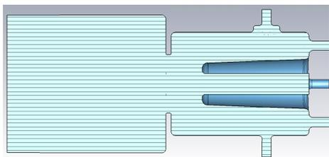
Figure 4: The enlarged tube HOM coupler.
