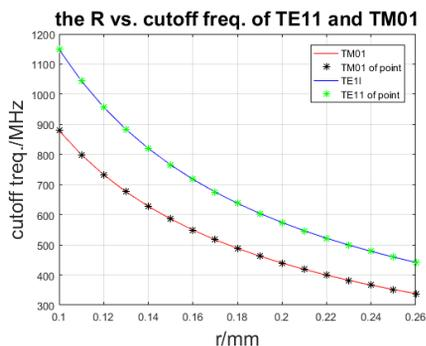
Figure 5: The cutoff frequency of TE11 and TM01 w.r.t. the tube radius.
