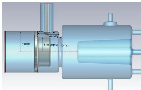
Figure 7: The coaxial-in structure.
