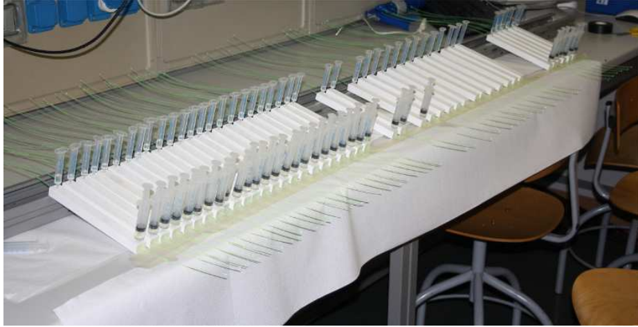
Figure 4.2: The WLS fiber gluing procedure.
