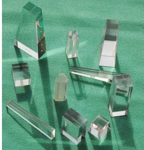
Figure 2.9: Several examples of different shapes of light guides used for the collection of the light produced in a scintillating plastic detector [53].
