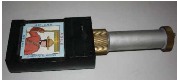
Figure 4.9: A photo of the scintillator for the trigger signal in the cosmic ray test of LEP.
