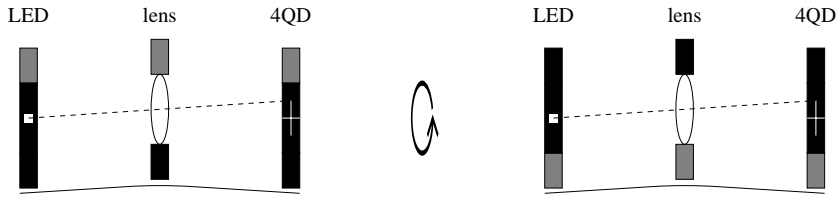
Figure 3.5 The effect of a displacement of the alignment stand at the lens position before and after rotation.
