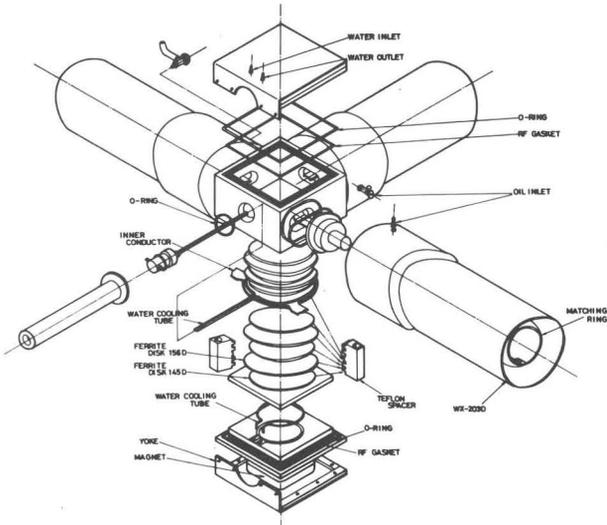
Fig. 2 Circulator assembly drawing
