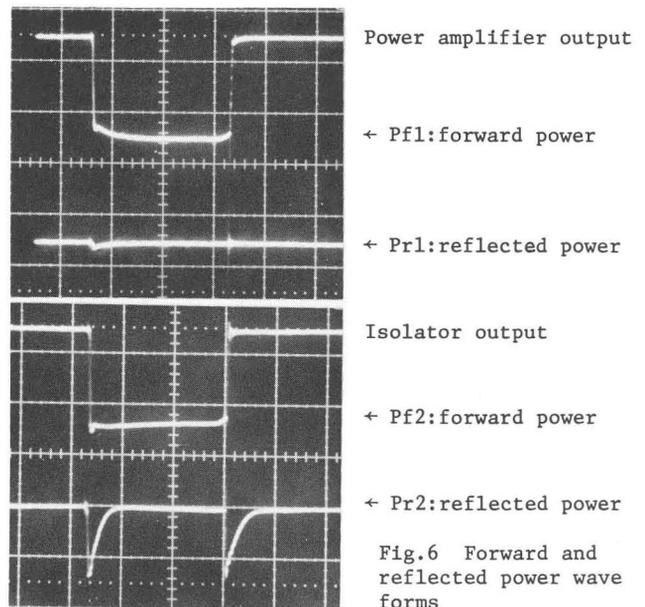
Fig. 6 Forward and reflected power wave forms
