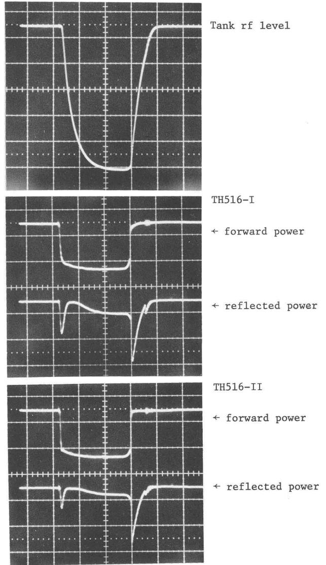
Fig. 8 Waveforms using isolators
