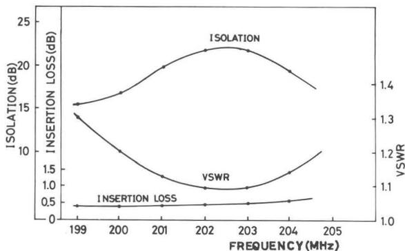
Fig. 4 Isolator characteristics
