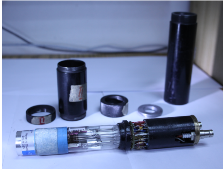
Figure 3.4: Detector housing, photomultiplier and BrillLance crystal.
