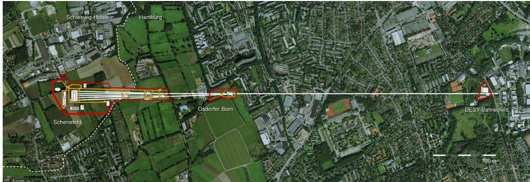
**Figure 2.2:** Birds-eye view of the future European XFEL, electrons will be accelerated from DESY-Bahrenfeld (right) in the direction of Osdorfer Born (middle) where undulators create the X-ray pulses that are then guided to the experiments in Schenefeld (left) (© European XFEL)
