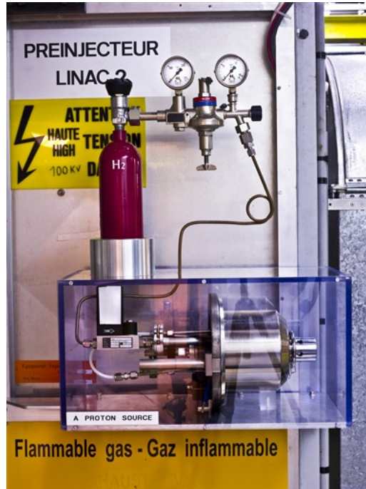
Figure 2.2: The source of protons for the LHC.
