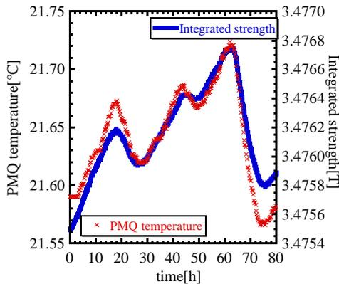
Figure 6: The weakest integrated strength vs time.
