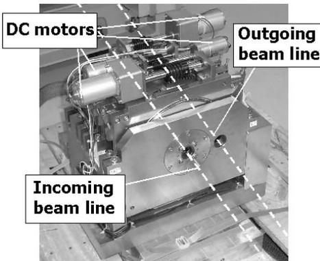
Figure 3: Fabricated 2<sup>nd</sup> prototype PMQ.
