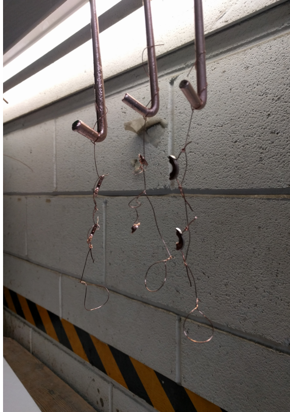
Figure 7.3: Split electrodes prepared for dipping in a bath at the commercial platers. These pieces were test pieces whose thickness was subsequently measured
