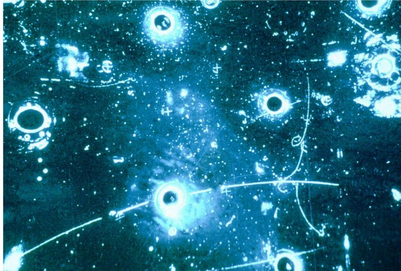
**Figure 5.4:** The first example of the neutral-current process  $\bar{\nu}_\mu + e^- \rightarrow \bar{\nu}_\mu + e^-$ . The electron is projected forward with an energy of 400 MeV at an angle of  $1.5 \pm 1.5^\circ$  to the beam, entering from the top.
