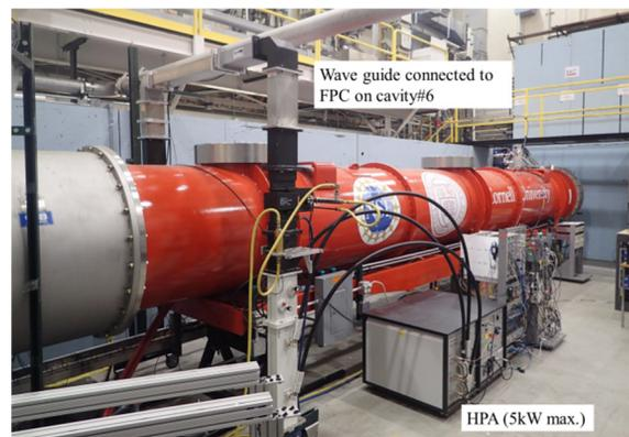
Figure 2: The MLC prototype in its final location.
