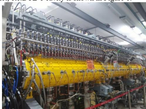
Figure 1: DTL-1 cavity situated in Linac tunnel.
