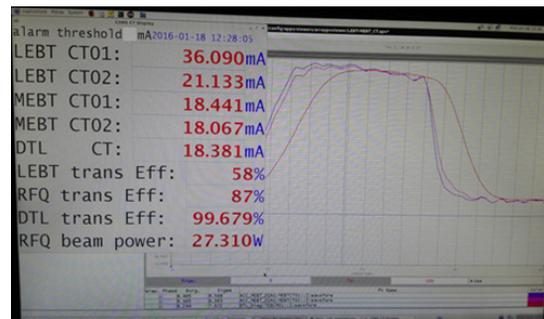
Figure 4: 18mA beam signal at the CT monitor.
