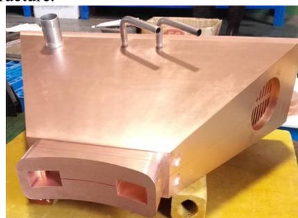
Figure 2: Ridge waveguide structure.
