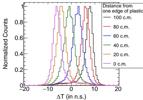
FIG. 3: Position information along a plastic bar from the timing response in the detector.
