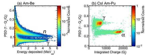
FIG. 1: PSD between neutron and  $\gamma$  in NE213 and between  $\alpha$  particles and  $\gamma$  in CsI(Tl).
