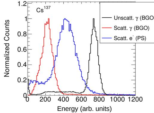
FIG. 4: Compton scattered  $\gamma$  and electron pulse height spectra from  $^{137}\text{Cs}$  in BGO and plastic.
