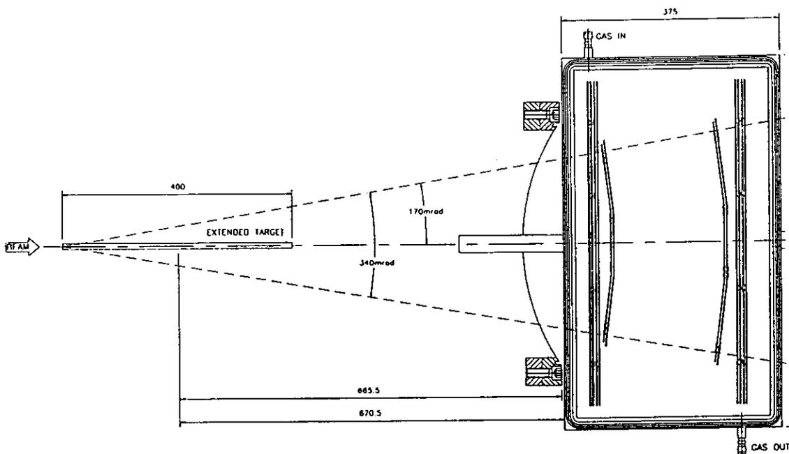
Figure 6.5: Set-up of the HERMES micro-strip gas counters (top view).
