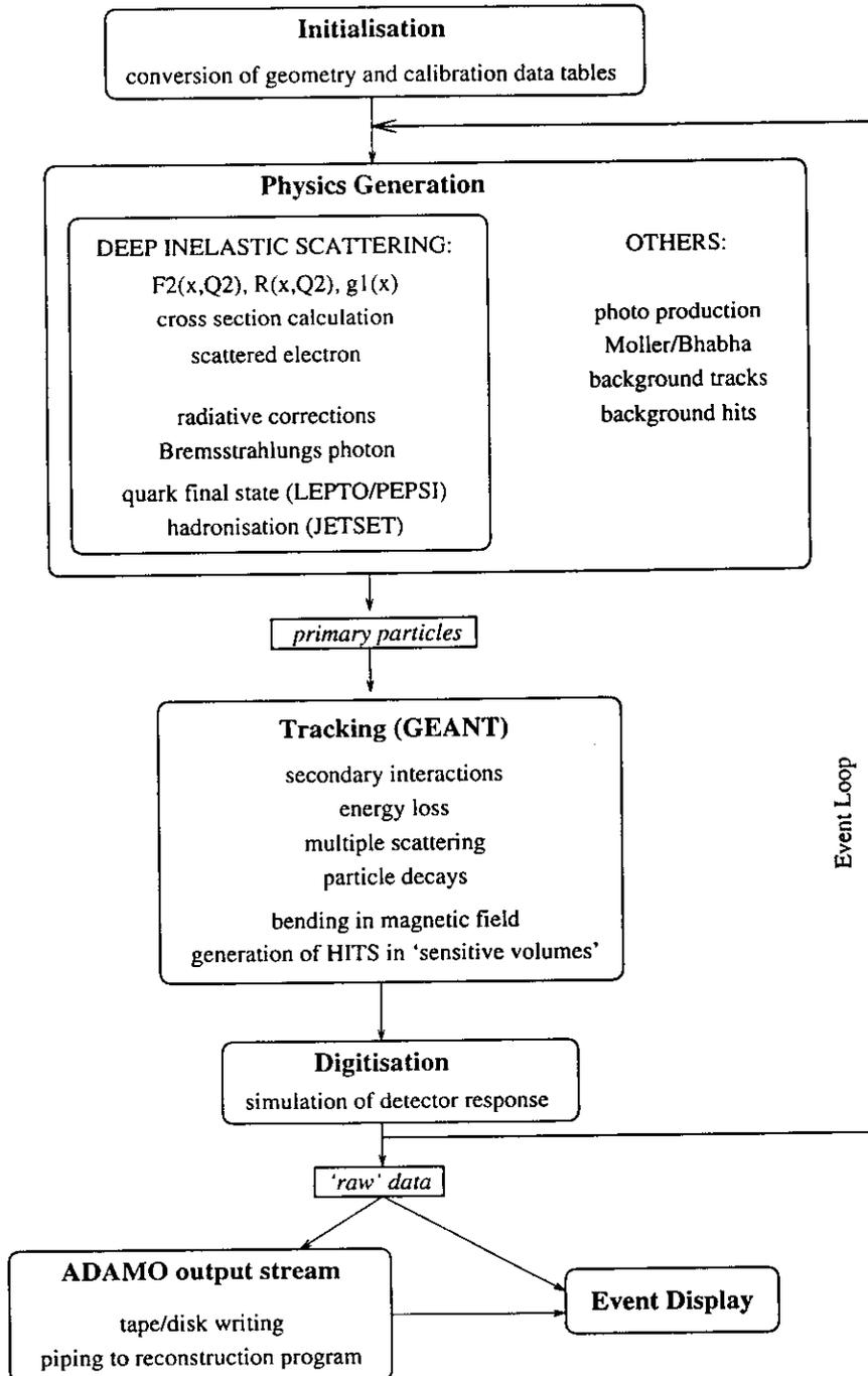
Figure 8.12: Simplified flow chart of the Monte Carlo program. The program has five main parts: the initialisation, the generation of the physics primary process, the tracking of the generated particles through the detector, the simulation of the detector response and the output of the information in ADAMO format. Single events may be visualised using the event display.
