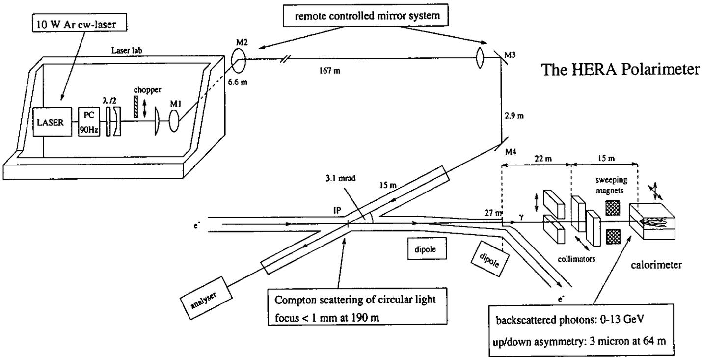
Figure 4.14: Layout of the HERA polarimeter. A laser beam is steered by a remote controlled mirror system into the HERA tunnel where it collides with the electron beam. Backscattered Compton photons are measured in a position sensitive calorimeter.
