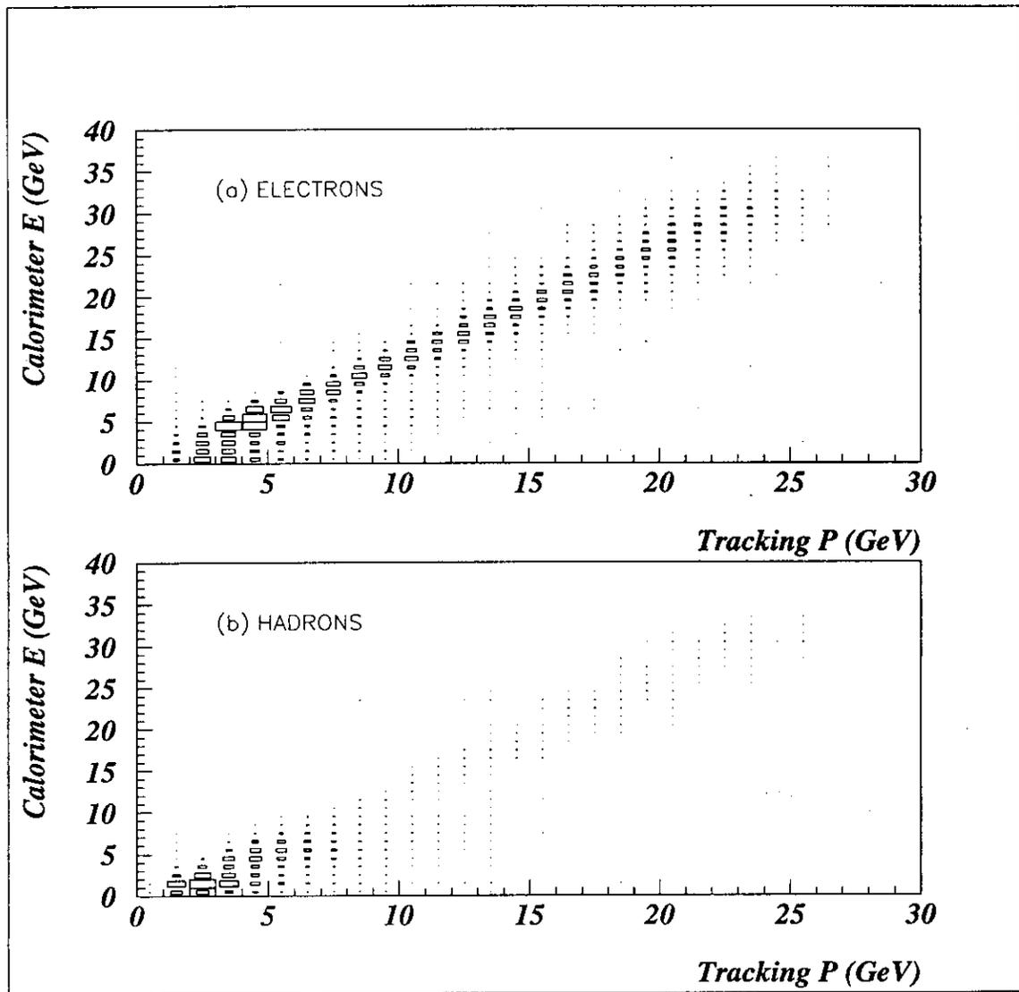
Figure 8.26: The energy of the cluster in the calorimeter is plotted versus the momentum of the corresponding track. Figure (a) contains all tracks which have a signal larger than 10 MeV in the preshower and figure (b) contains the rest of the tracks. This way electrons and hadrons can be separated to some extent. The band in figure (a) can be used to calibrate the calorimeter scale. The band in figure (b) comes from misidentified positrons.
