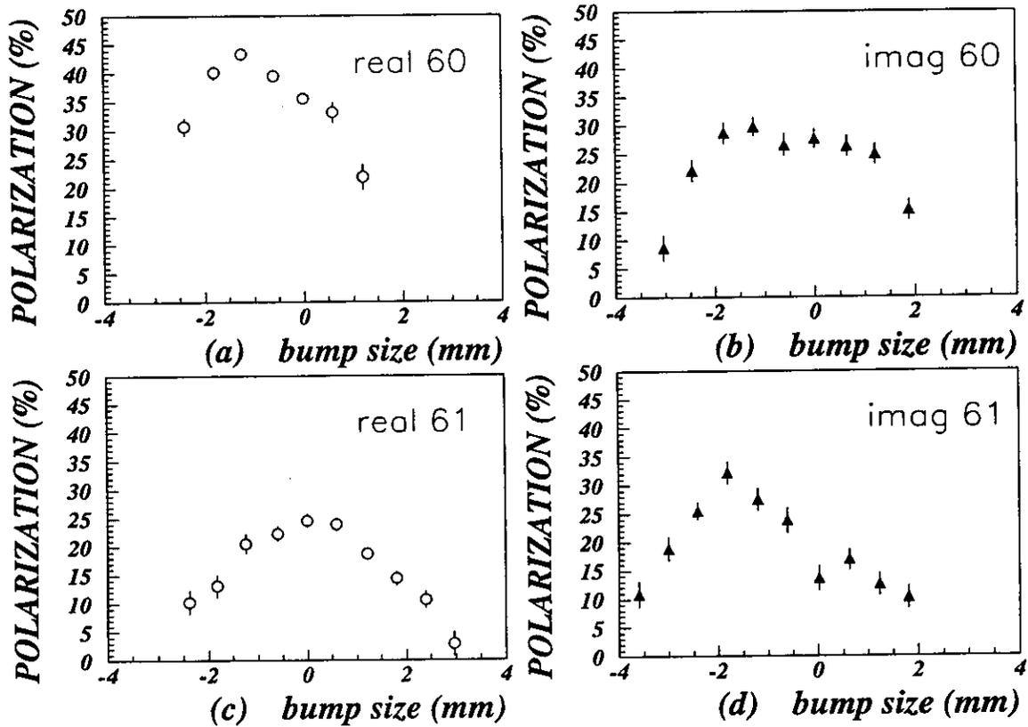
Figure 4.2: Scan of four harmonic corrections bumps. The polarisation is plotted versus the maximal orbit deviations due to the bumps. The plots are not corrected for rise time effects. The figure shows that polarisation strongly depends on the amplitude of the bumps. Polarisation is optimised by finding the maximum of the curve for each harmonic.
