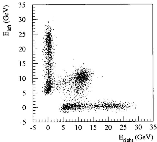
Figure 8.21: Plotted is the energy deposit in the left versus the right luminosity counter. The bands are mainly due to Bremsstrahlung background in one of the counters. The patch in the middle shows a clear signal of Bhabha scattering. The sum of the energies in the counters is approximately the beam energy of 27.5 GeV. Part of the showers is lost due to the limited apertures of the crystals. The trigger threshold is 5 GeV.
