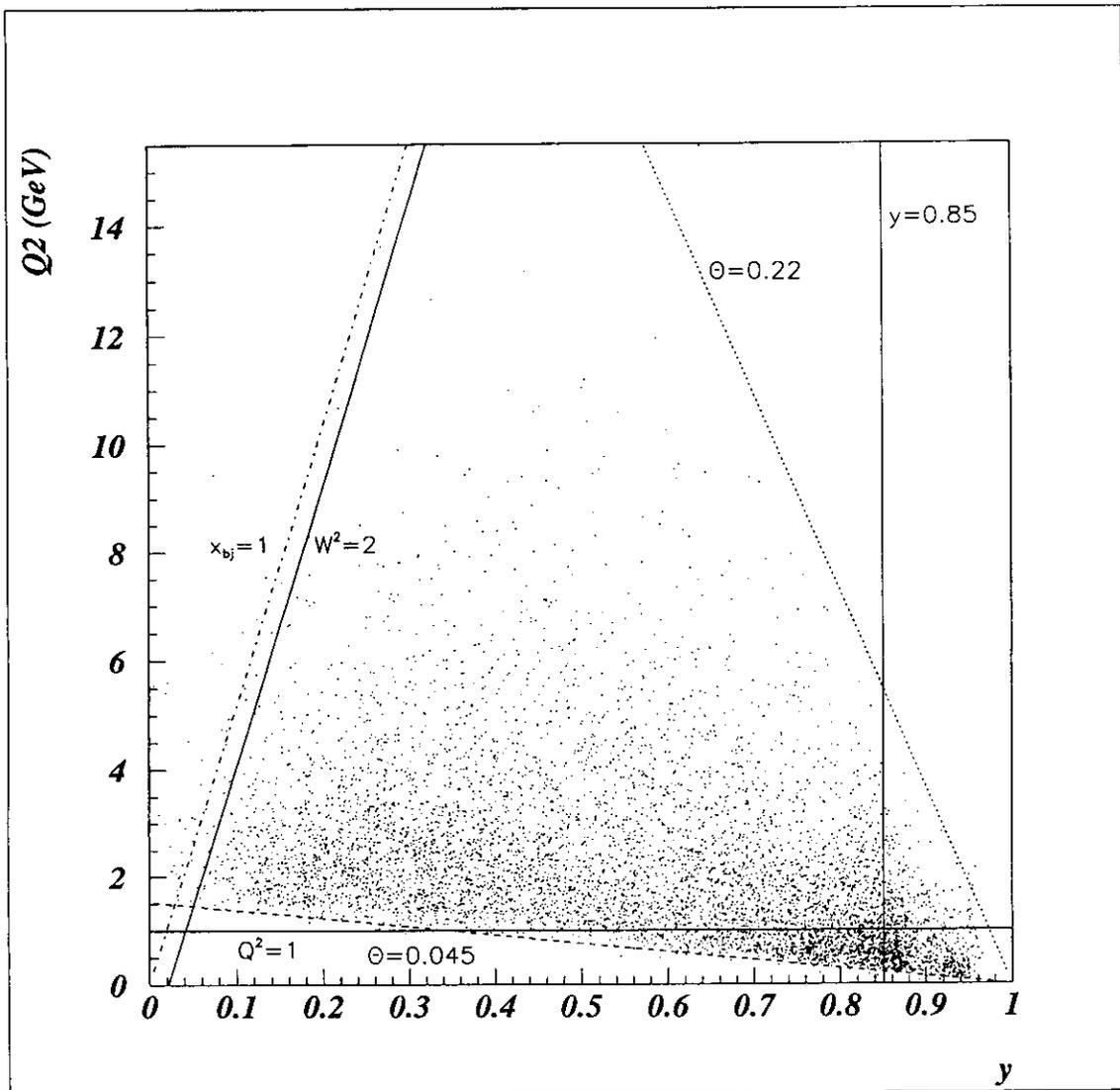
Figure 8.29: The distribution of real data events in the kinematic plane is shown. According to the deep inelastic cross section the highest population is at low  $Q^2$ .
