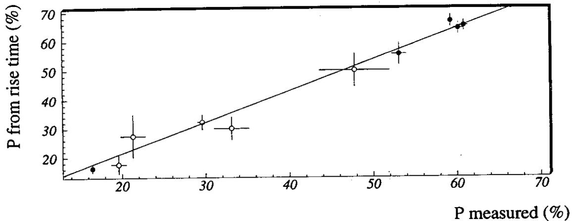
Figure 4.26: Comparison of the polarisation extracted from the rise time constant compared to the measured value in the polarimeter. The two values agree within the statistical and systematic uncertainties.
