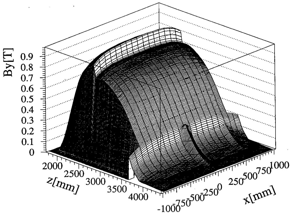
Figure 6.3: Measured field map of the HERMES spectrometer magnet for  $I = 950$  A at  $y = 96$  mm.
