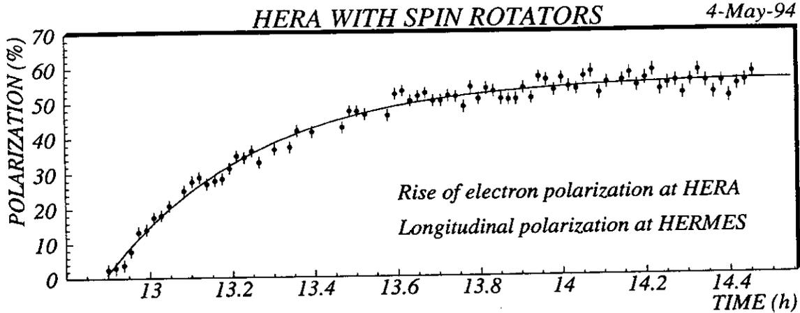
Figure 4.7: First observation of longitudinal polarisation at HERA. Overlaid is the result of a fit of the expected exponential build-up curve with the parameters  $P_{\infty} = 56.6 \pm 0.5\%$  and  $\tau = 20.8 \pm 0.7$  min.
