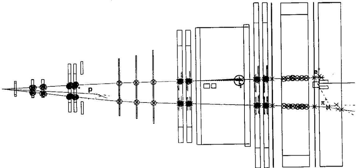
Figure 8.13: Top view of a Monte Carlo generated deep inelastic event.
