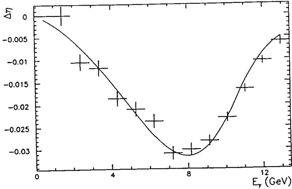
Figure 4.24: The shift of the means  $\Delta\eta$  plotted as function of the energy of the backscattered photons. The shape agrees well with the predicted analysing power. From the fit (solid curve) an polarisation value of  $P_e = 53\%$  has been extracted.
