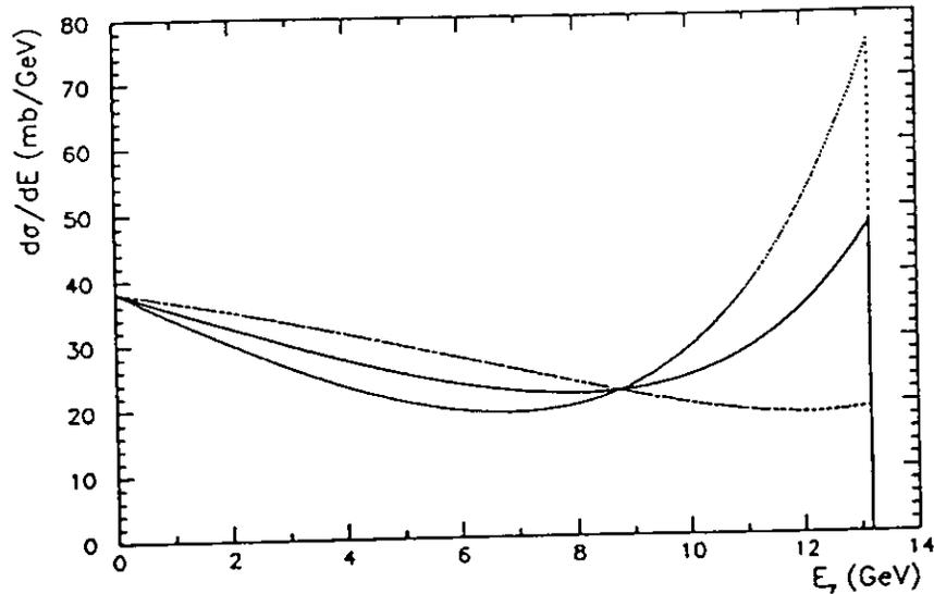
Figure 4.13: The energy spectrum of the backscattered Compton photons is shown for the case that the electrons are unpolarised (solid curve), longitudinally polarised with  $S_3P_z = 1$  (dashed curve) or longitudinally polarised with  $S_3P_z = -1$ .
