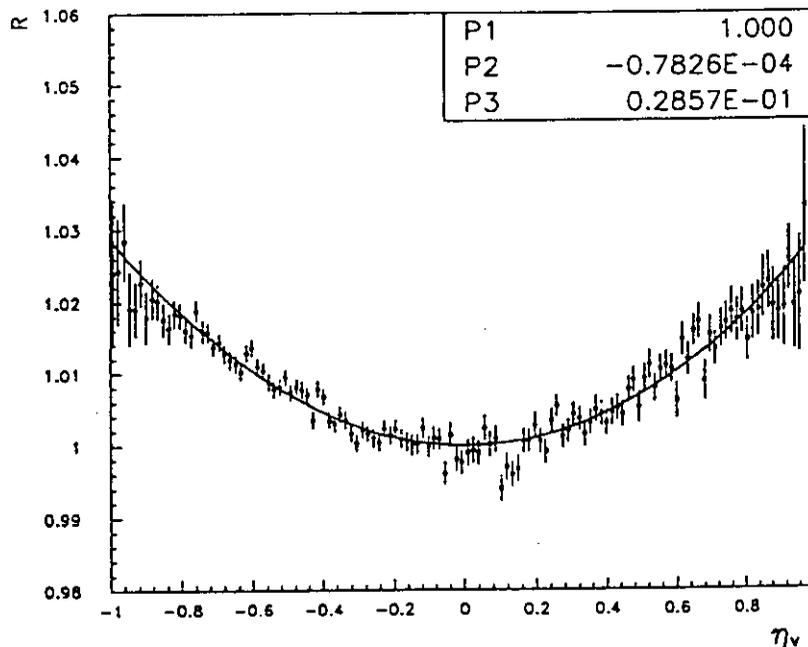
Figure 4.19: The ratio  $R$  of the 'vertical energy' divided by the 'horizontal energy' is plotted as function of  $\eta$ . The calorimeter is properly calibrated as the fit  $R(\eta) = P_1 + P_2\eta + P_3\eta^2$  gives  $P_1 = 1$  and  $P_2 = 0$ .
