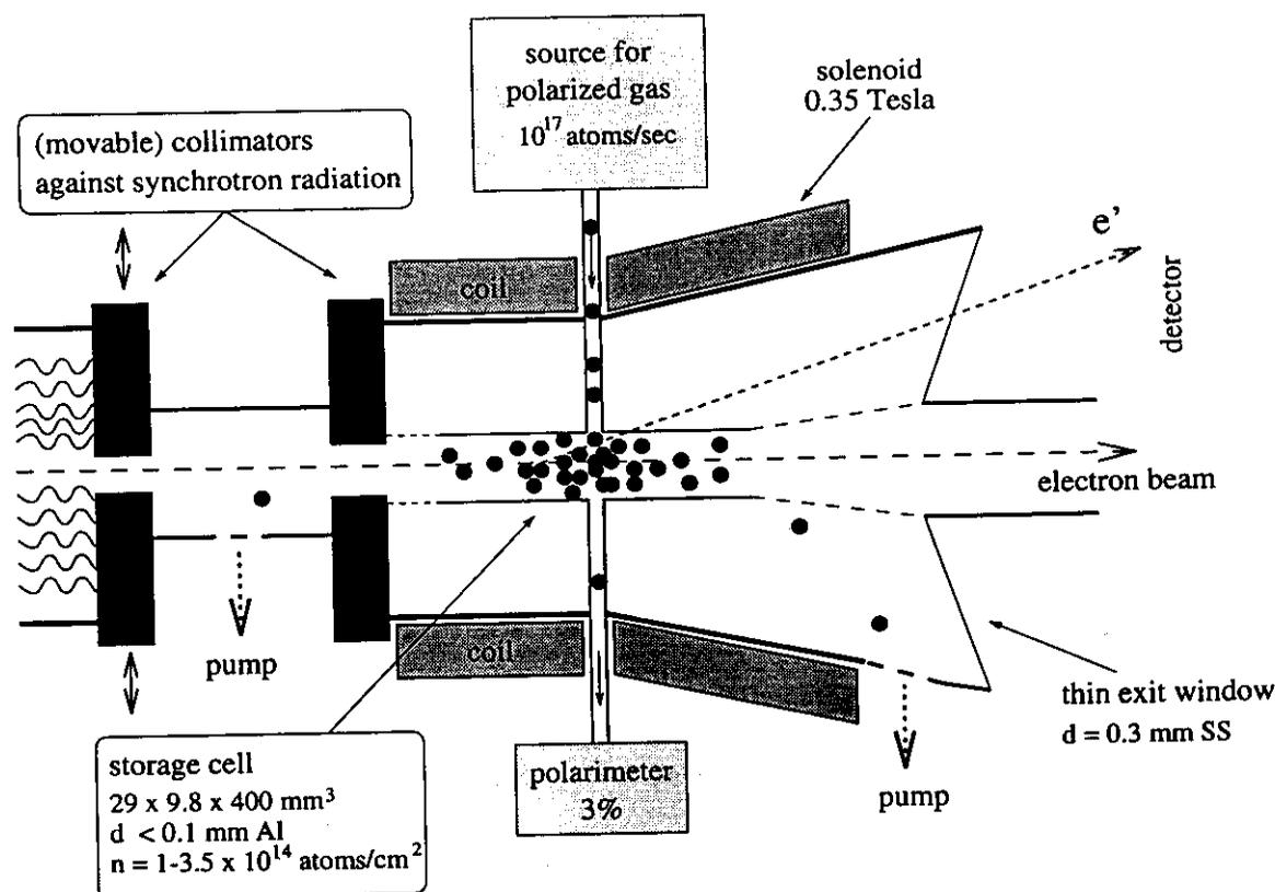
Figure 5.6: Simplified sketch of the HERMES target region. The storage cell is protected against synchrotron radiation and beam tails by a collimator system. Rf-meshes protect from electromagnetic fields. Large pumps keep the vacuum conditions good despite of the target gas leaking out of the storage cell.
