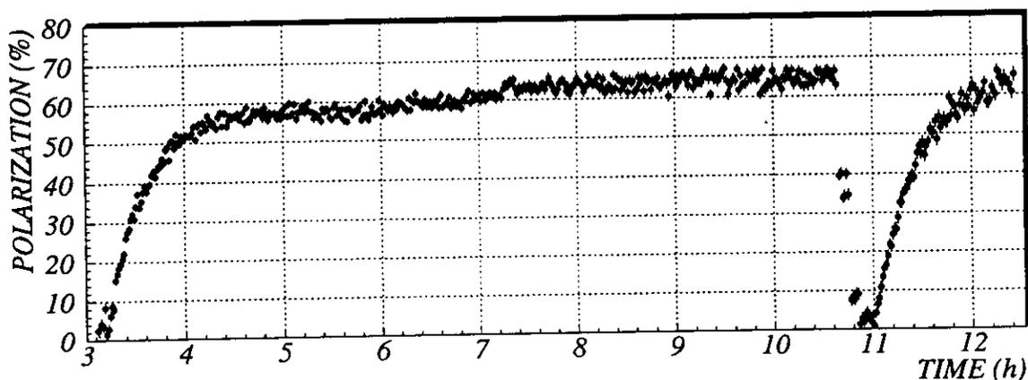
Figure 4.9: Polarisation during a long luminosity run. The polarisation rose after ramping the beam to 27.5 GeV. At 6:00 it is likely that beam conditions changed slightly which led to an increase of polarisation. At 10:30 the beam was depolarised by rf-resonance to perform an energy calibration and to cross check the polarimeter calibration. At 12:30 the beam was dumped.
