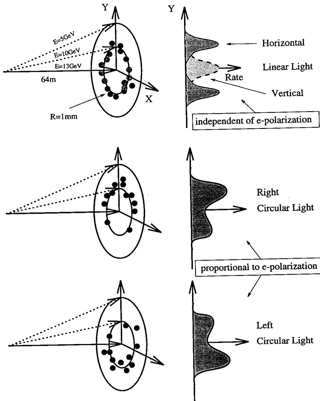
Figure 4.12: Backscattered Compton photons of a fixed energy arrive at the detector in a circle with defined radius. The detector measures the vertical projection of the Compton distribution. For linear light, the distribution is an even function of  $y$  and independent of the electron polarisation. For circular light the distribution has an odd component which is proportional to the transverse electron polarisation. This effect is used to measure the transverse polarisation.
