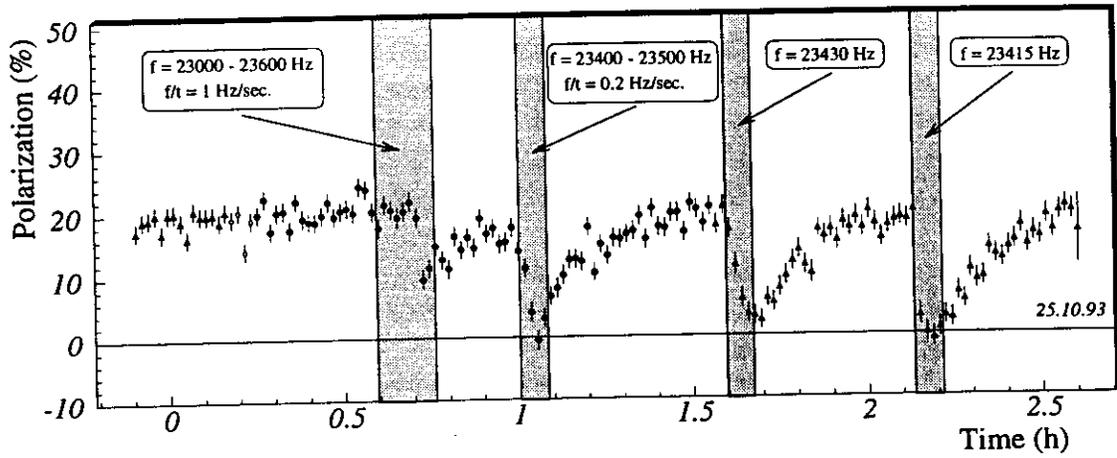
Figure 4.10: Resonant depolarisation of the HERA beam using different frequencies and sweeping speeds. The efficiency of the depolarisation depends on the amplitude of the magnetic field and on the speed of the frequency sweep. The depolarisation frequency is found by tracing back the frequency from the moment at which depolarisation occurred and by iteratively reducing the sweeping ranges. Unlike at LEP, spin-flip could not be observed at HERA.
