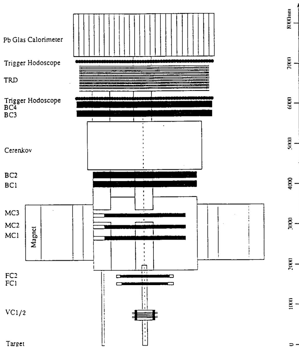
Figure 6.4: Schematic view of the arrangement of the different detector components.
