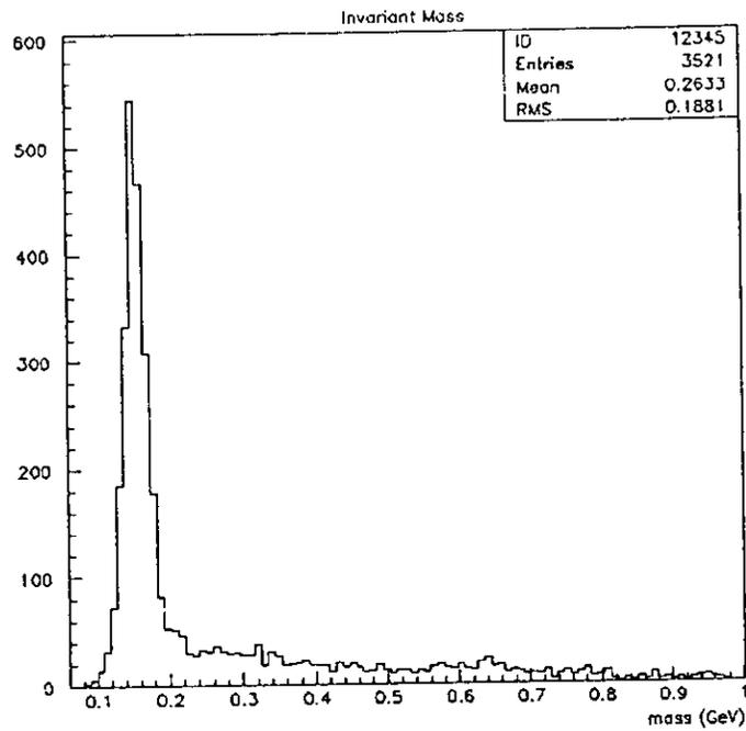
Figure 8.5: Plotted is the invariant mass of two photon clusters in the calorimeter. The abscissa is not calibrated. At 0.157 a clear  $\pi^0$  peak is seen. At 0.640 there is a small peak of the  $\eta^0$ .
