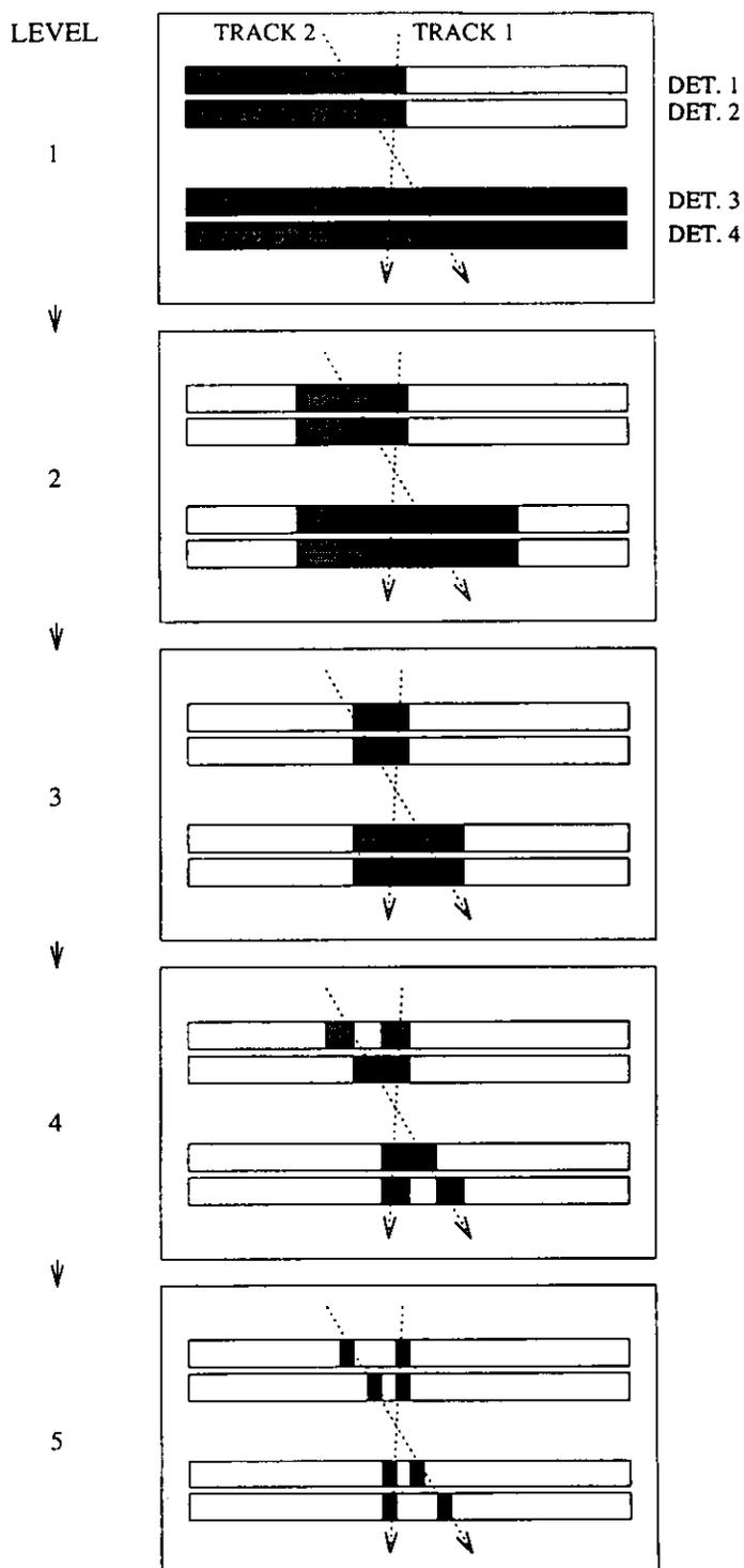
Figure 8.9: The tree search algorithm looks at the hits of the tracking detectors with artificially reduced resolution. In every tree search level the resolution is doubled until a resolution is reached which is optimal for track finding. The optimal resolution is determined by the resolution of the chamber plus some alignment uncertainties.
