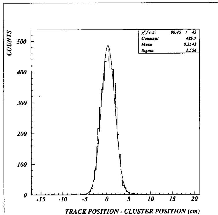
Figure 8.25: Clusters in the calorimeter are correlated with tracks. The granularity of the calorimeter is 9 cm. The position of the centre of a cluster is reconstructed from the relative energy sharing between neighbouring cells. The figure shows that the centre of the clusters agrees with the position of the extrapolated track within a resolution of  $\sigma = 1.6$  cm.
