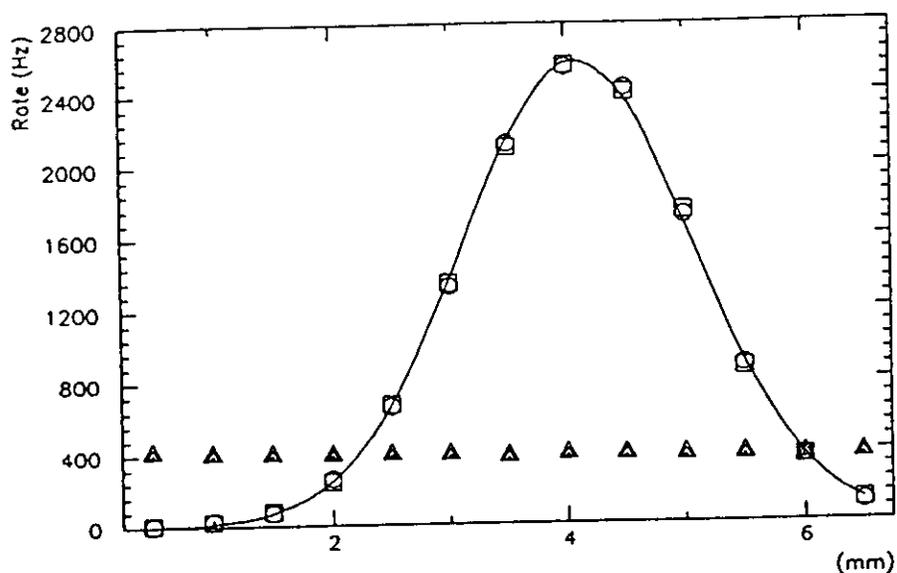
Figure 4.15: The combined width of the laser and electron beam are measured by scanning the laser beam across the electron beam. The circles (squares) show the Compton rate for left (right) polarised circular light. The RMS-width is 1 mm and the shift between the two polarisation states is compatible with zero ( $2 \pm 8 \mu\text{m}$ ). The triangles show the background rate which decreases slightly due to the decay of the electron current over the time of the scan.
