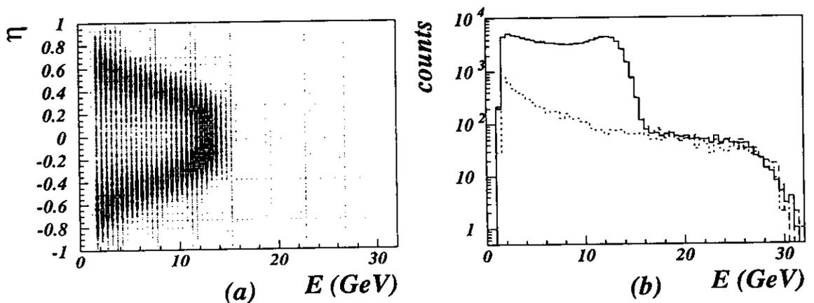
Figure 4.18: The two-dimensional distribution (position  $\eta$  versus energy) of the backscattered Compton photons (a) and its one-dimensional energy projection (b) for the two cases that the laser is on (full line) or off (broken line). The Bremsstrahlung background is suppressed by more than a factor of 10 compared to the Compton rate. The Compton edge at 14 GeV is used for the energy calibration of the calorimeter.
