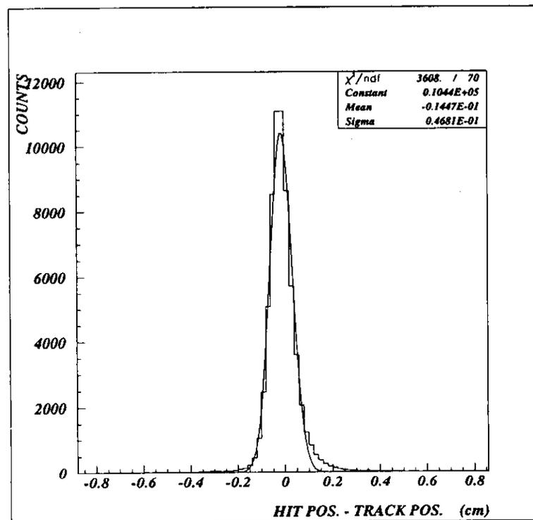
Figure 8.4: Plotted is the residual of the tracks compared to the position measured in the backward drift chambers. The current value of  $\sigma = 0.47 \text{ mm}$  will be further optimised by a more precise alignment and calibration.
