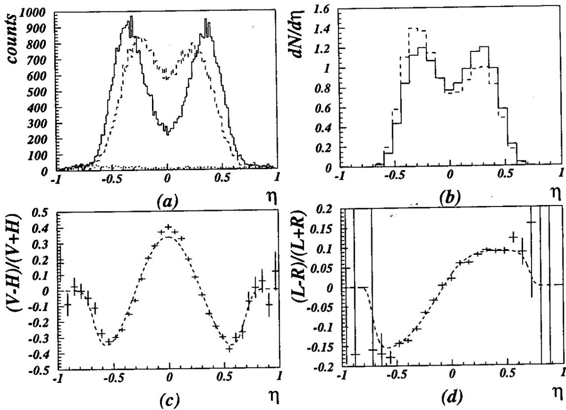
Figure 4.23: The  $\eta$ -distributions for Compton scattering off horizontal and vertical linear (a) polarised light and right and left circular (b) polarised light and its asymmetries (c) and (d). The lower plots are derived from the upper distributions. The even component of the asymmetry curve is proportional to the linear light asymmetry (c) and the odd one is proportional to the product of circular light polarisation and electron polarisation (d).
