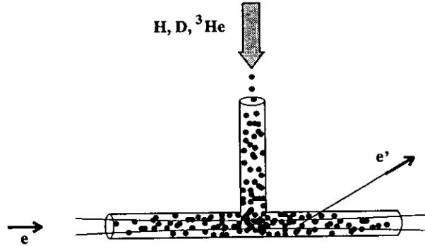
Figure 5.2: Principle of the storage cell target. The atoms are injected into a T-shaped tube and perform several hundred wall bounces before they leave the cell. This way the thickness of a gas target is increased by two orders of magnitude compared to a free gas jet.
