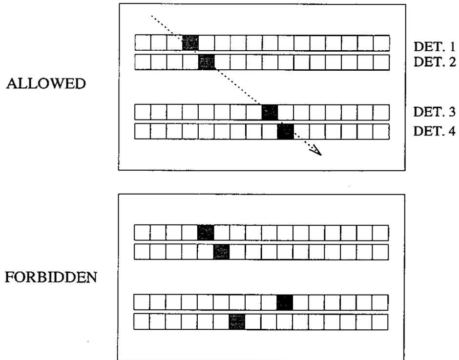
Figure 8.10: At each tree search level, the allowed and forbidden pattern are well defined. The program compares the measured pattern with the data base and finds out if the measured pattern contains a pattern of an allowed track. Symmetry considerations allow to reduce the number of different allowed pattern in each level to a number which can be handled by the computer.
