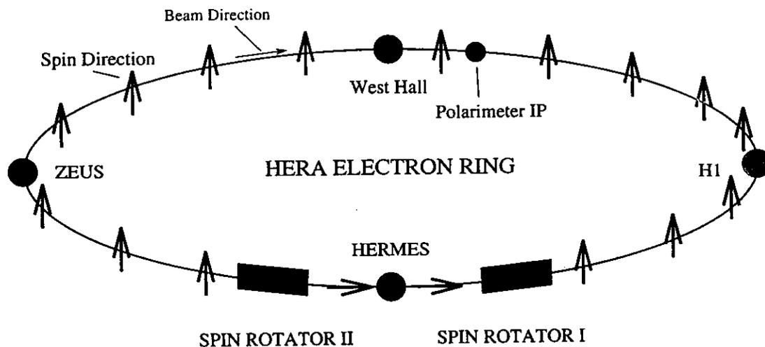
Figure 4.4: A sketch of the HERA electron ring showing the positions of the spin rotators. Polarisation is longitudinal in the straight section at the HERMES IP. Transverse polarisation is measured with the Compton polarimeter in the West area.
