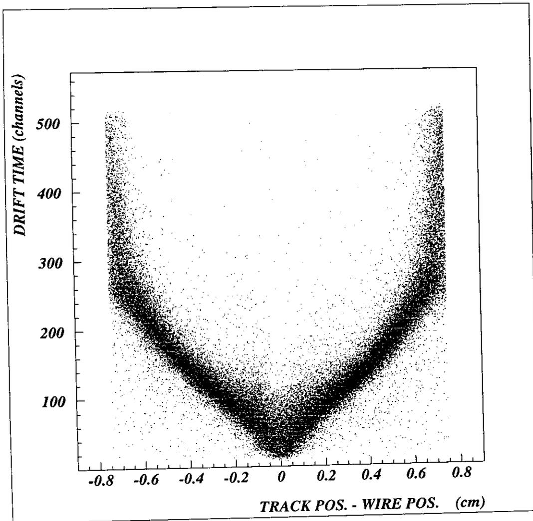
Figure 8.3: Shown is the drift time versus the distance of the reconstructed track to the nearest sense wire for the backward drift chambers. One channel in the TDC corresponds to 0.5 ns. The 'V' plot is a multi-purpose plot. It can be used to extract alignment constants,  $T_0$ 's, SDTR's and the resolution of the detector.
