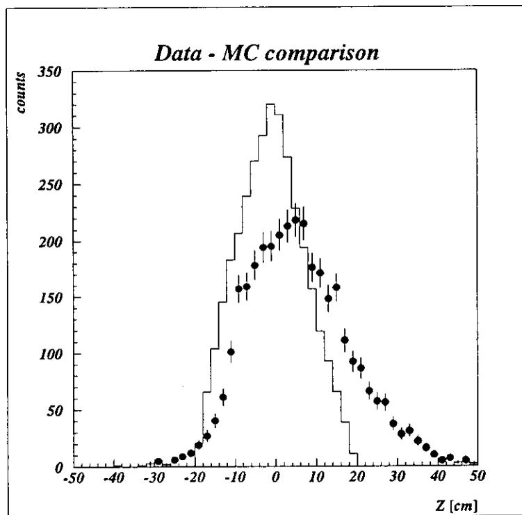
Figure 8.24: Plotted is the longitudinal vertex distribution. Due to the present mechanical deformation of the cell the vertex distribution is no longer triangular. The shift and the smearing of the distribution is mainly due to the fact that the alignment and calibration of the chambers is not finished yet.
