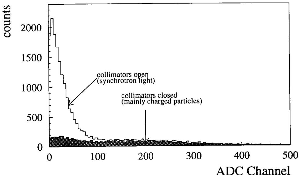
Figure 8.22: Shown is the ADC spectrum of a silicon counter behind the target window which is sensitive to synchrotron light. When the movable collimators are open and only one elliptical fixed collimator protects the cell, a peak at low energy deposit is observed which is caused by synchrotron light. The peak completely disappears when the movable collimators were closed.
