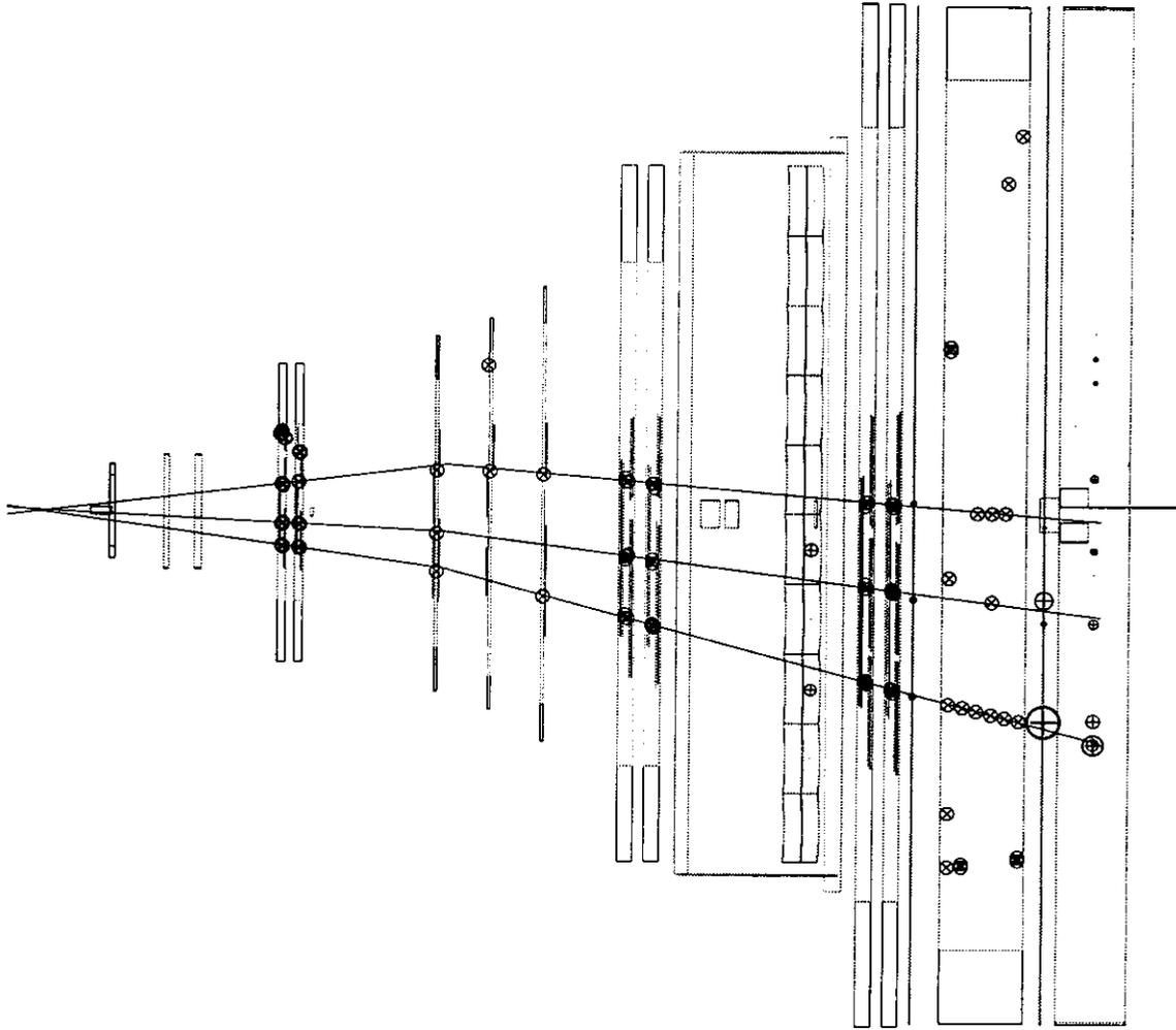
Figure 8.31: The plot shows a top view of an event with three tracks and a common vertex.
