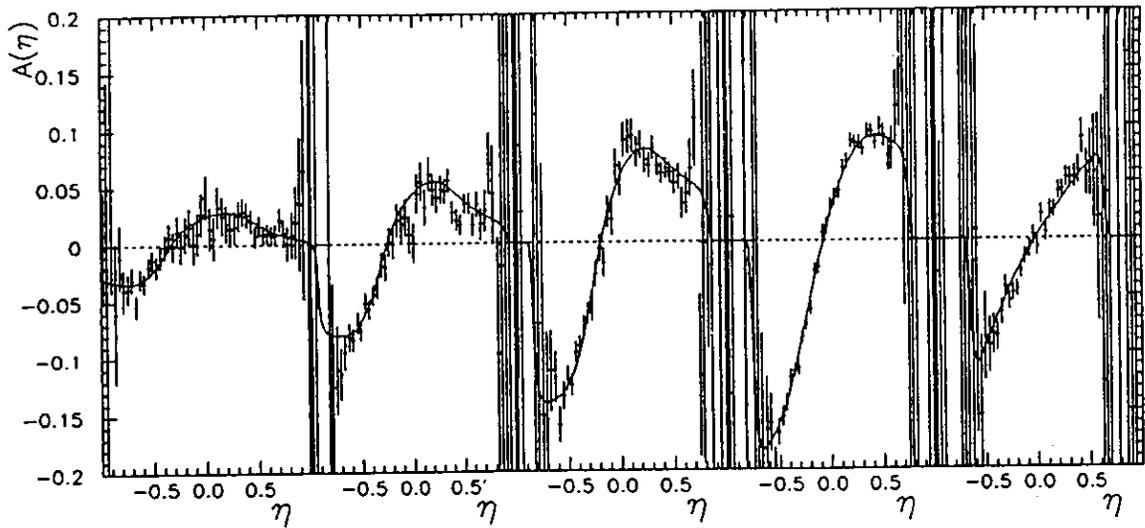
Figure 4.22: The asymmetries  $A(\eta)$  are shown for the same energy intervals as in the previous figure. A simultaneous fit gives an electron polarisation of  $P_e = 54.8 \pm 0.7\%$  and a linear component of the light of  $\Delta S_1 = 8.8 \pm 0.4\%$ .
