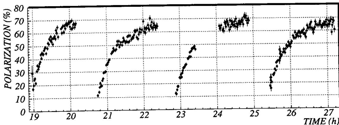
Figure 4.8: Recording of longitudinal polarisation during HERA bake-out runs. After each injection and ramping of a new beam, the polarisation rises exponentially and reproduces high values close to  $P = 70\%$ .
