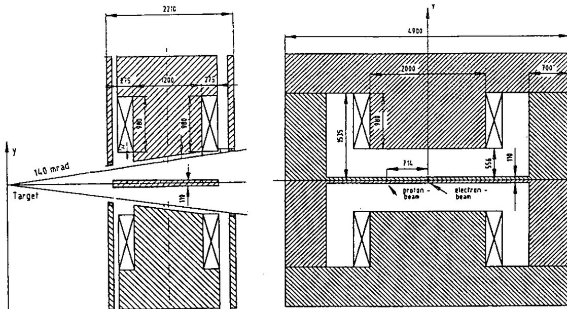
Figure 6.2: Layout of the HERMES spectrometer magnet with septum plate (side and front view).
