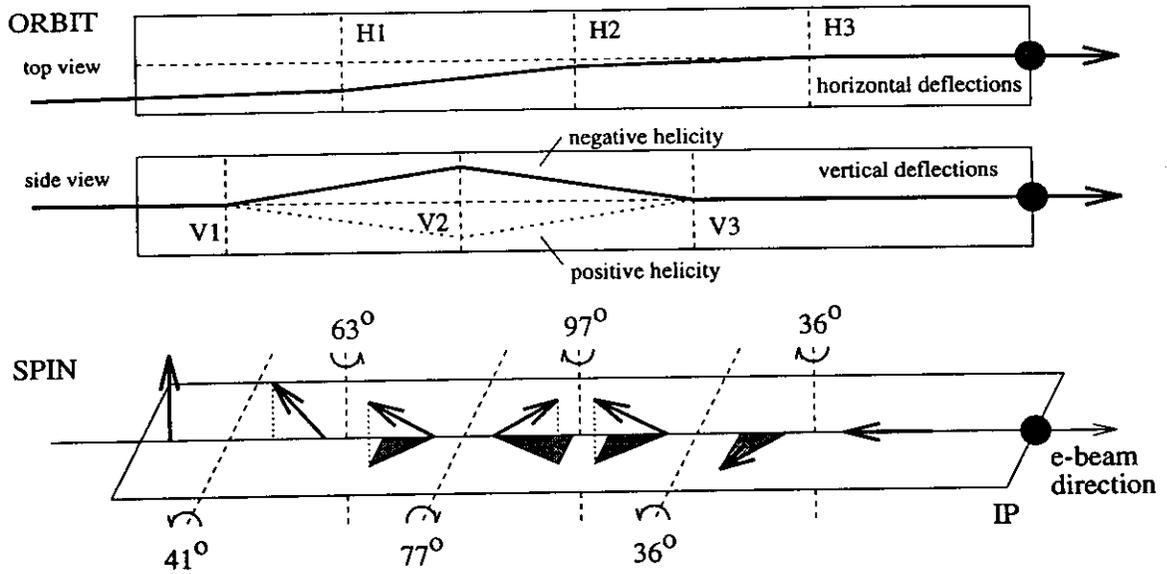
Figure 4.6: A functional diagram of the Mini-Rotator showing the horizontal and vertical deflections of the orbit and the corresponding spin precession angles. The size of the vertical bump is about 22 cm. The spin precession is a factor of 63 larger compared to the orbital kicks. Due to the non-Abelian behaviour of rotations, it is possible to rotate the spin by  $90^\circ$  and at the same time move the orbit back to its nominal position and slope.
