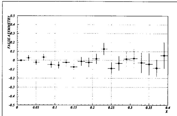
Figure 8.30: The data from a 50 minute run have been split into two parts ( $A$  and  $B$ ). A false asymmetry  $(A - B)/(A + B)$  which is formed from the two subsets is compatible with zero. It illustrates the size of the statistical errors which can be expected for the polarisation measurements.
