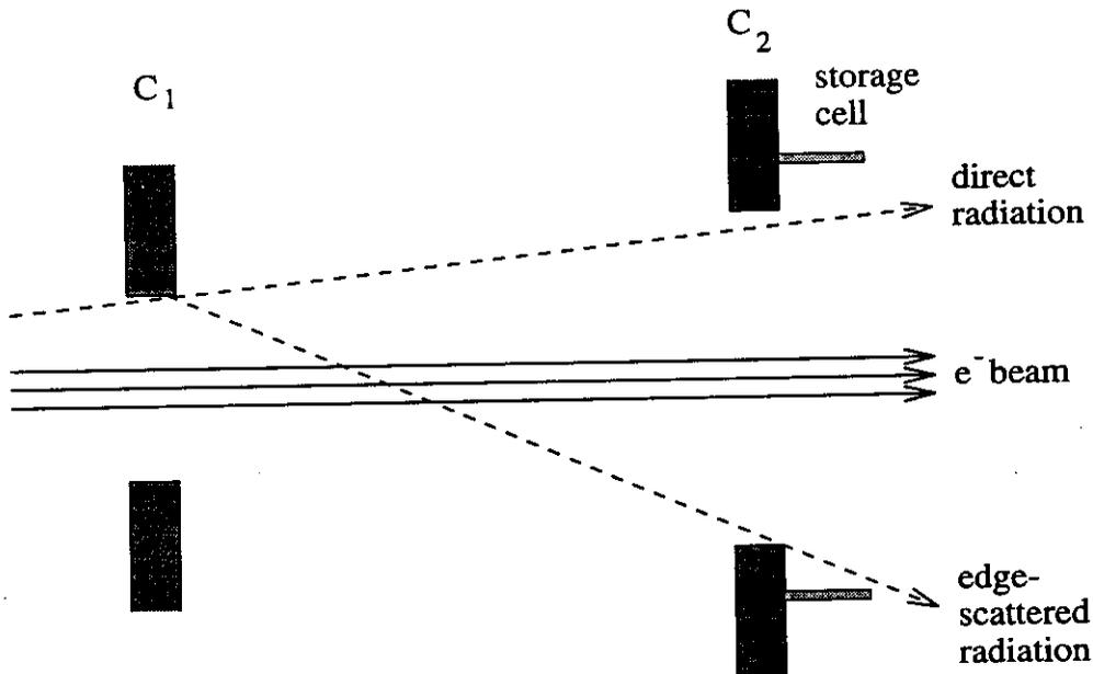
Figure 5.5: Sketch of the collimator system.  $C_2$  is in the shadow of direct synchrotron radiation. The storage cell and the detector are in the shadow of direct radiation and of radiation that is edge scattered at  $C_1$ .
