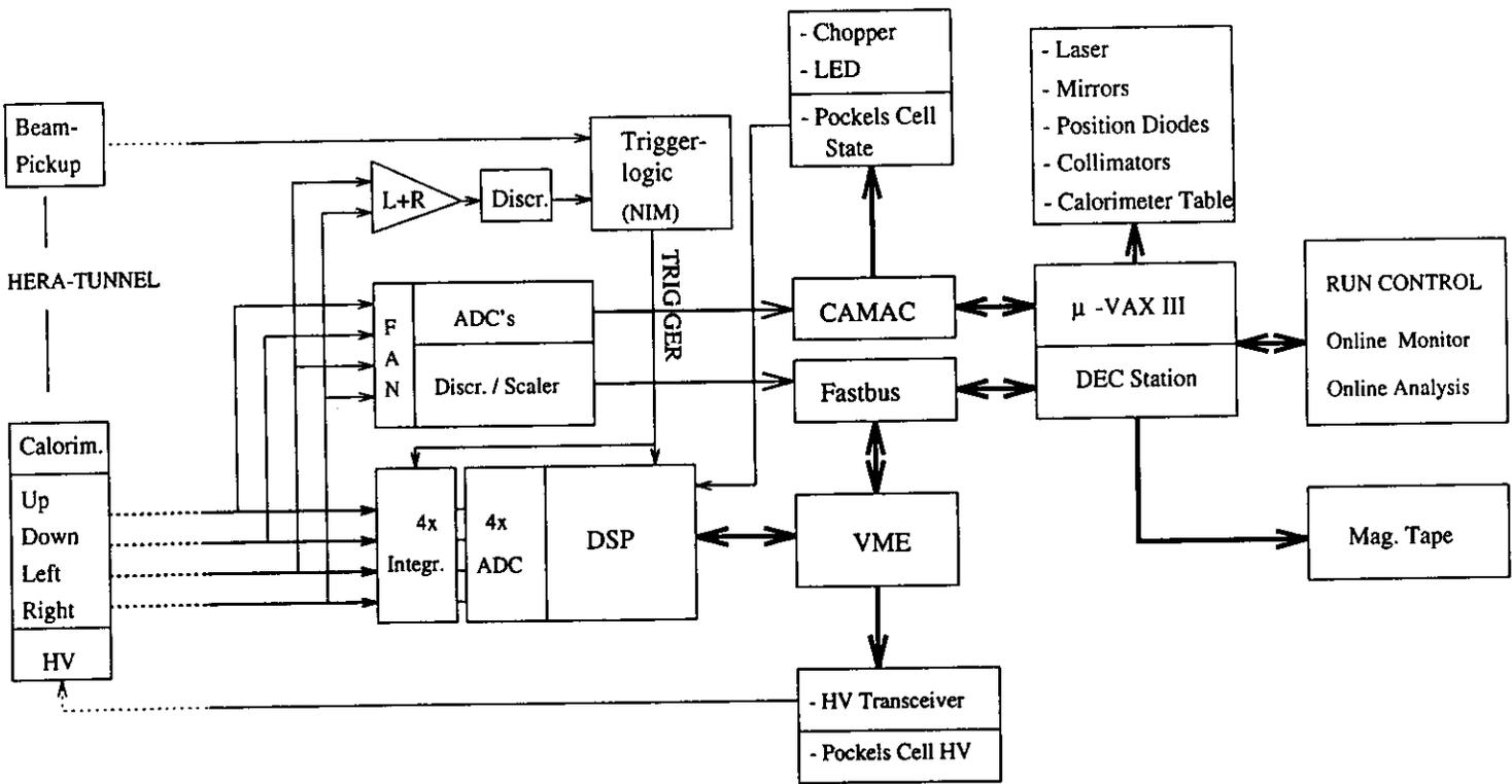
Figure 4.20: An overview of the polarimeter DAQ system.
