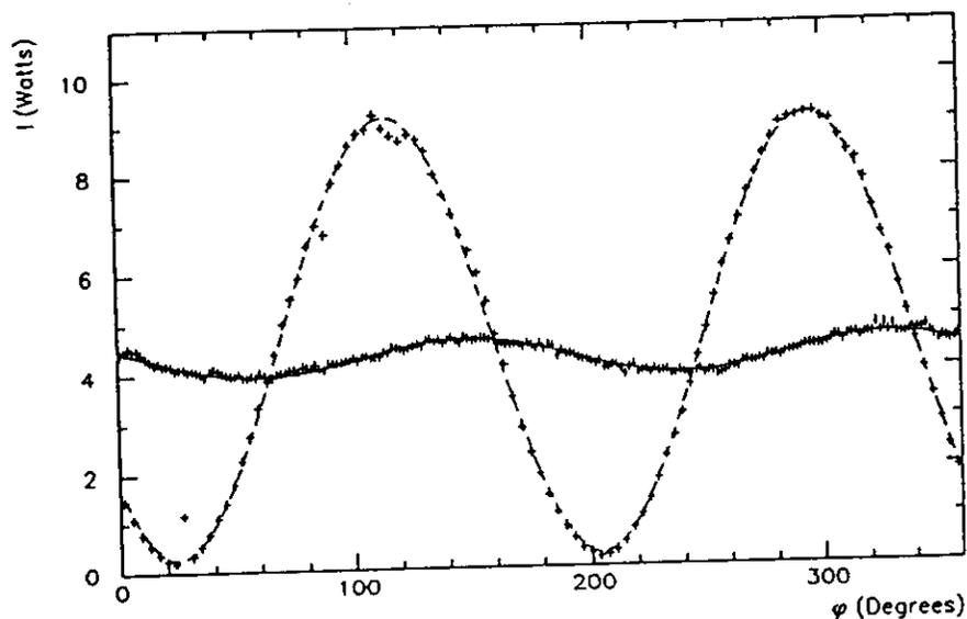
Figure 4.16: The degree of linear and circular polarisation is measured by analysing the intensity of the light versus the orientation of the Glan prism. The fits correspond to a linear polarisation of 94% for the case the Pockels cell is off (broken line) and 8.5% for the Pockels cell on (solid line). The remnant linear component of 8.5% corresponds to a degree of circular polarisation of 99.6%.
