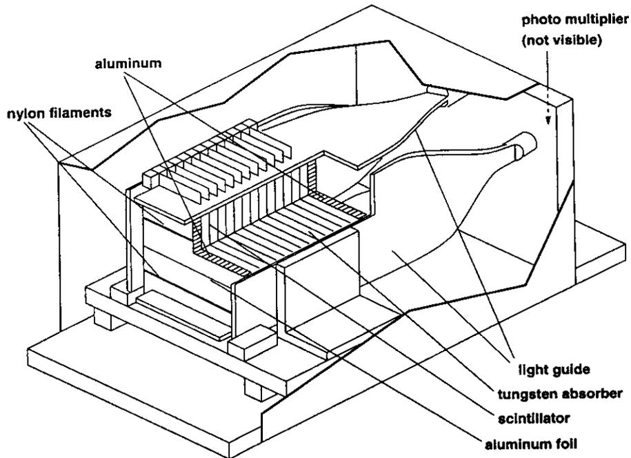
Figure 4.17: A cutaway, perspective view of the tungsten scintillator calorimeter is shown. The calorimeter has an upper and a lower half which are optically decoupled. The scintillating light is collected by wavelength shifters on all four sides. The asymmetry of the shower development in the upper and lower half is used to measure the vertical projection of the impact point of the photon.
