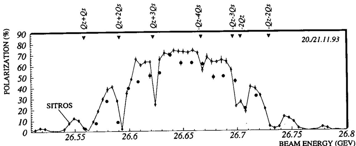
Figure 4.3: Comparison of the measured (dark dots) versus the calculated polarisation at HERA as a function of beam energy. Two side-band resonances could be measured (at 26.59 GeV and 26.71 GeV). The bell-shaped behaviour of polarisation versus energy is reproduced. The absolute value of polarisation depends on the quality of the harmonic bump optimisation.
