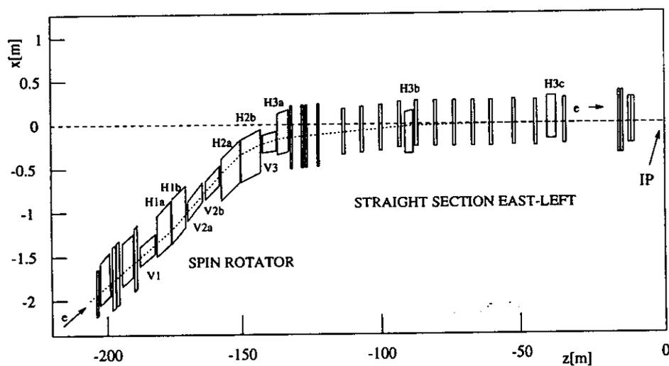
Figure 4.5: Horizontal projection of the layout of one  $90^\circ$  spin rotator. H1-3 (V1-3) indicate the horizontal (vertical) bending dipoles of the Mini-Rotator. The thin boxes indicate quadrupoles.
