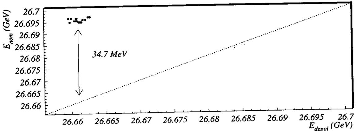
Figure 4.11: The beam energy of HERA was calibrated by rf depolarisation. The 'true' beam energy was found to be 33-36 MeV below the nominal beam energy which is calculated from the dipole currents. The deviation is within the systematic uncertainties of the dipole fields.
