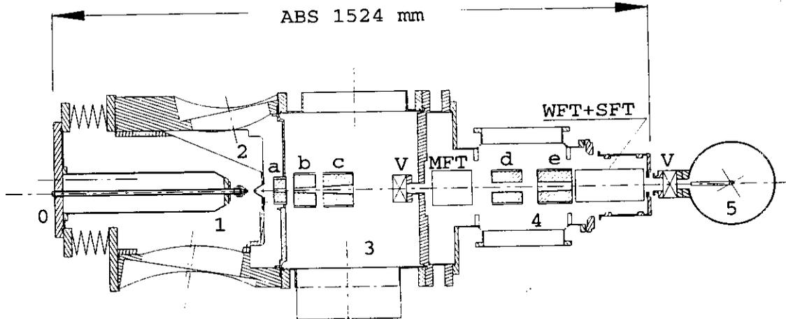
Figure 5.1: Sketch of the polarised atomic beam source for HERMES. The dissociator is in chamber 1. A beam is formed and focussed by the sextupole magnets a-e. MFT, WFT and SFT denote medium, weak and strong field transitions. The atomic beam is injected in the storage cell in chamber 5. The chambers can be separated by valves (V).
