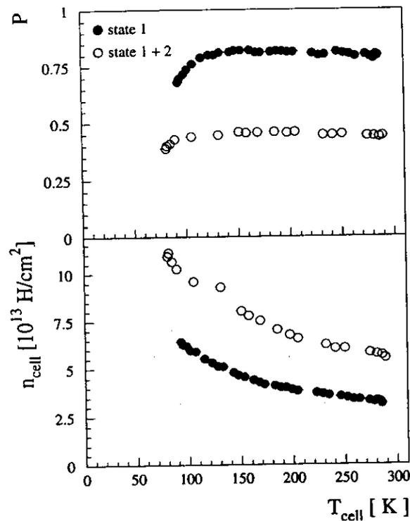
Figure 5.3: Polarisation and thickness of the gas in the storage cell as a function of cell temperature. The polarisation drops only at very low temperatures (upper plot) due to wall depolarisation. The target thickness is higher at low temperatures as the atoms need more time to leave the storage cell (lower plot). In these measurements only a weak magnetic field could be applied to the target resulting in a maximum polarisation of  $P_{max} = 0.5$  when using two hyperfine states.
