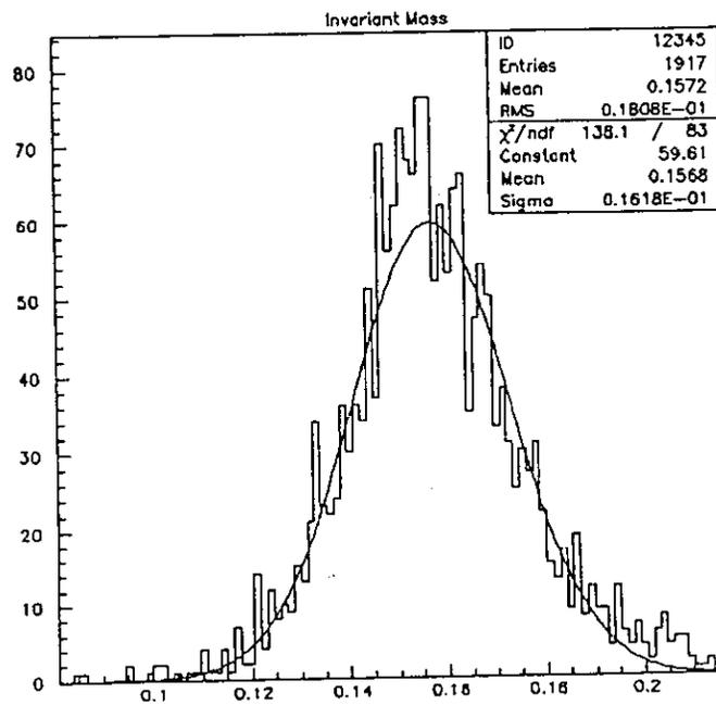
Figure 8.6: A blown-up scale of the  $\pi^0$  peak shows that the scale of the abscissa is off by 16%. The true value of the  $\pi^0$  mass is 135 MeV.
